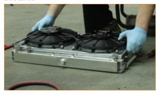
2. Place radiator into the vehicle, making sure to secure it on the radiator mounting peg holsters.
