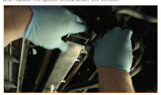
5. Replace the upper radiator hose and securely tighten the hose clamps.
