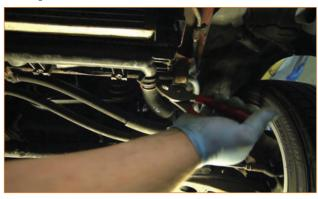
5. Using your ratchet, remove the two 10mm bolts securing the air conditioning line to the vehicle.
