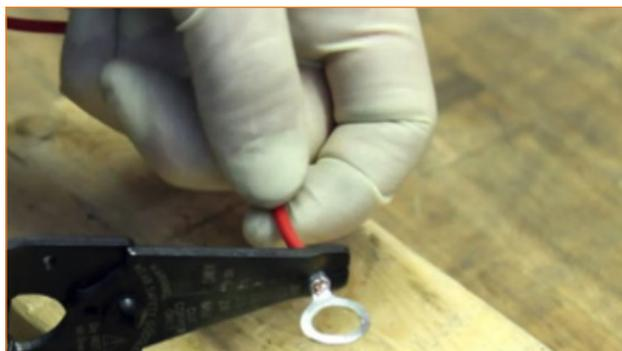
19. Slide the shrink tubing over the base of the ring connector and use a heat source to melt the shrink tubing. Be sure the tubing covers any exposed wire.
