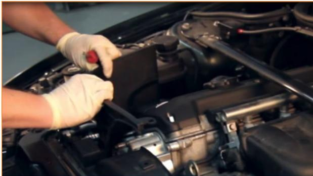
8. Remove the electrical connector. Set the connector aside until needed later.
