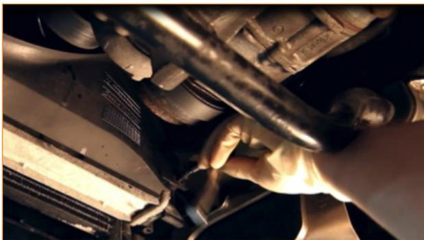
11. Remove the screws from the upper fan shroud. (2x T25 Torx screws)
