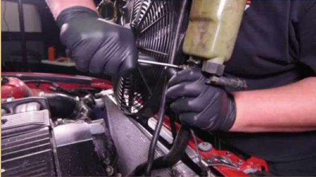
**19.** Install the supplied bracket for the stock expansion tank. (2x 10mm bolts)
