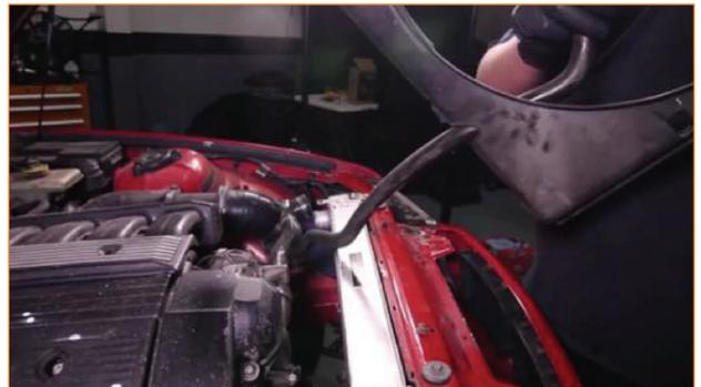
16. Install the rubber bushings onto the Mishimoto fan shroud. (4x bushings and 2.5mm Allen bolts)
