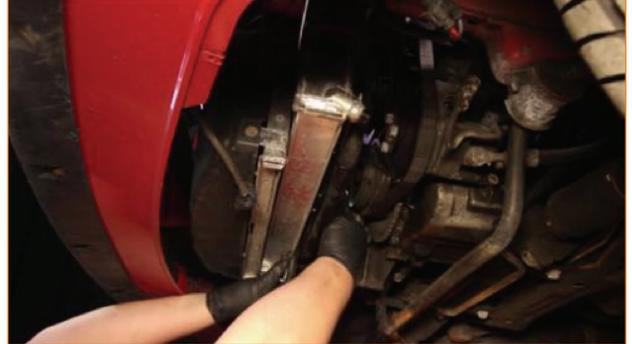
**25.** Reinstall the air dam using the Phillips head screws and pop clips removed in **step 1**.
