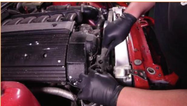
11. Unseat the stock expansion tank and feed the overflow hose out of the way.
