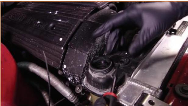
10. If the Mishimoto X-line E36 Performance Radiator is already installed, run the overflow line through the shroud. (Depending on the radiator model, routing the line may be slightly different)
