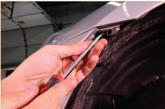
13. Remove the ten pop-clips that secure the splash shield to the bottom lip of the bumper cover. (10x pop-clips)
