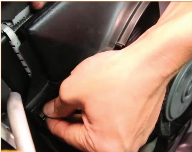
24. Prep the Mishimoto fan shroud. Attach the provided plate to the two-bolt flange near the bottom of the fan shroud, but do not fully tighten. (2x 10mm bolts)
