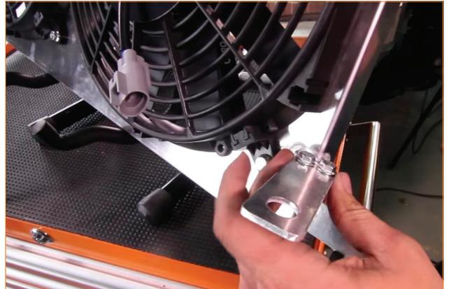
25. There are two holes along the upper edge of the fan shroud. Install the long dowel to the hole closest to the corner of the fan shroud, but do not fully tighten. Install the short dowel to the hole farthest from the corner on the fan shroud, but do not fully tighten. (2x 10mm bolts, 2x dowels)
