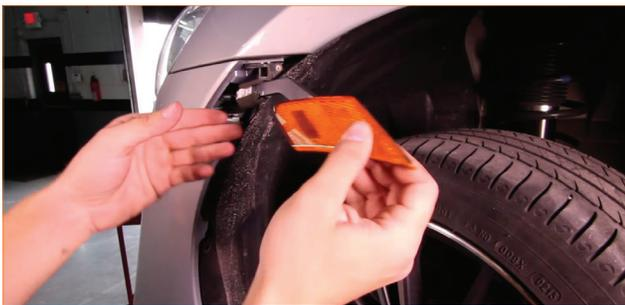
12. Remove the pop-clip behind the side marker light; it connects the bumper cover to the fender. Do this on both sides. (2x pop-clips)
