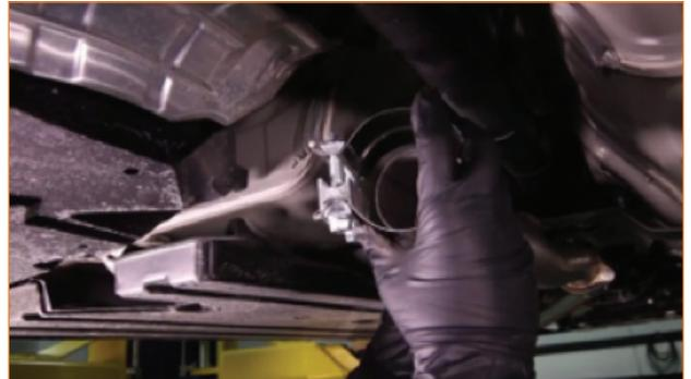
6. Spray the rubber exhaust hanger with WD-40 and attach to the Y-pipe.
