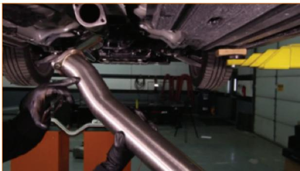
4. Make sure that all five of the rubber bushings for the exhaust hangers are properly in place, and then attach the two mufflers. Spray the hangers with WD-40 to help them slide into place.
