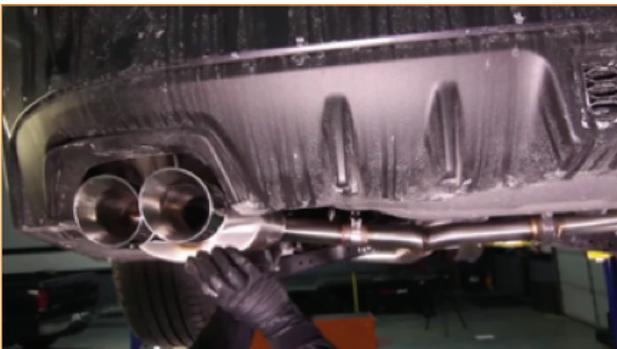
10. Tighten the mid-pipe to Y-pipe band clamp. (14mm deep socket, 14mm wrench)
