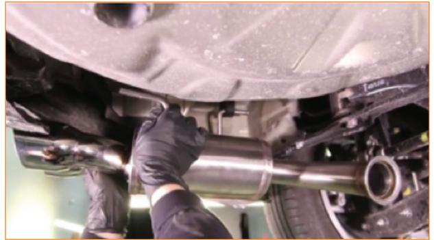
5. Install the band clamp exhaust onto the mid-pipe. Make sure the hardware faces the driver side.
