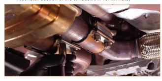
**04.** Remove the two bolts that secure the exhaust hangers to the rear subframe. Lift the exhaust and unhook the hangers from the rear subframe. (2x 13mm bolts)
