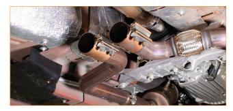
10. Slip the Mishimoto X- or H-pipe into the clamps on the exhaust, but do not tighten them yet. When properly installed the M emblem on the exhaust brace should be right side up.
