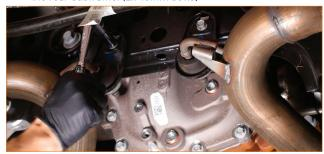
**05.** Support the exhaust system with a jack stand. Pry back the tab on the exhaust clamp, and slide the clamp back toward the resonator. Do this on both clamps.
