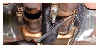
06. At this point the exhaust will be held in with only the rear hangers, so be prepared to handle the weight. We recommend having a friend help with removal. Lubricate the rear hanger grommets, and slide the exhaust system forward until the hangers are free of the grommets.
