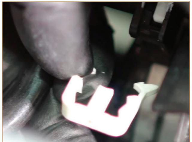
12. Disconnect the vacuum line from the intake manifold by depressing the white tab and sliding the connector off the manifold.
