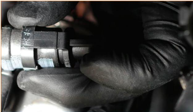
18. Separate the throttle body wiring harness clip from the throttle control motor by pushing it off.
