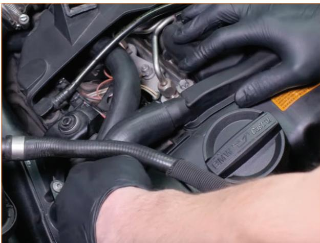
12. Loosen the bolt that secures the back of the coolant reservoir and remove the bolt in the front. (2x 10mm bolts)
