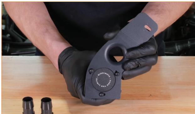
02. Install the provided fittings to the catch can and snug them down with a wrench, but do not overtighten them. These fittings have a tapered thread so they will not be flush with the can when fully installed.
