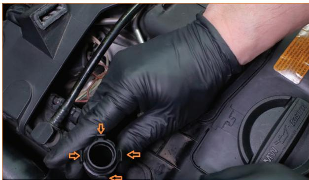
07. Remove the CCV hose and heater element by pulling the heater directly out of the intake tube.
