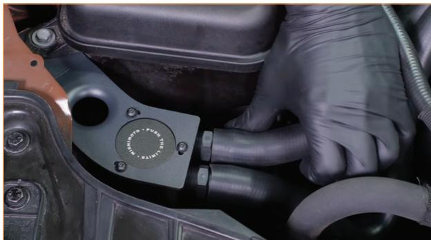
15. Adjust the catch can hoses so that they run tightly along the valve cover. This ensures that the engine cover will fit nicely. Now go back and tighten the bolts that secure the catch can to the bracket.
