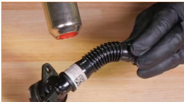
09. Reinstall the heater to the intake tube and secure it with the two Torx screws. Then reconnect the electrical harness. (2x T25 Torx screws)
