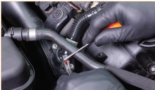
05. Remove the two Torx screws that secure the heater element to the intake tube. (2x T25 Torx screws)
