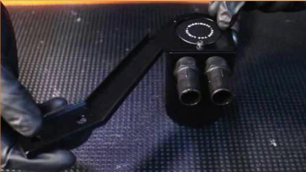
21. Remove the two 10mm nuts from the bracket that holds the power steering reservoir in place.
