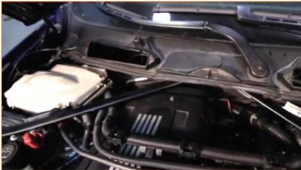
12. Remove the four Allen bolts on the engine cover, and then remove the cover from the engine bay.
