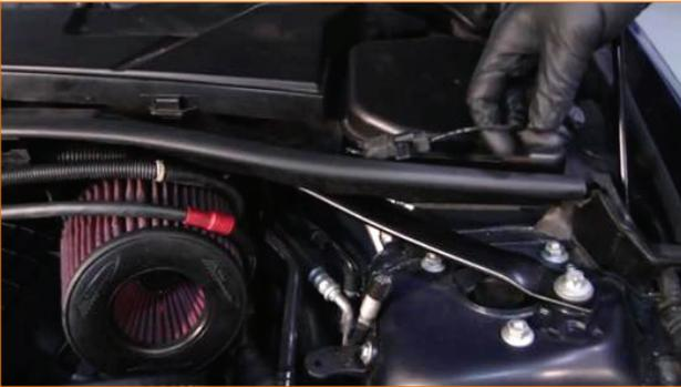
6. Twist the harness on the passenger side about 30 degrees and pull outward. Set the harness aside.
