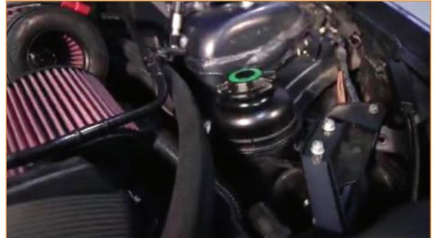
23. Connect the hose coming from the valve cover to the inlet on the catch can. (These hoses are under vacuum, so worm-gear clamps are not required.)
