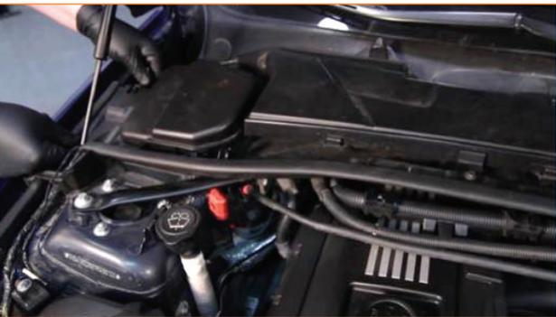
8. Remove the driver-side panel by lifting up on the two side tabs and moving the last tab toward the cabin of the vehicle.
