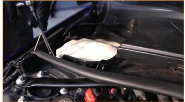
10. Remove the six 8mm course-threaded bolts that hold the cabin filter to the main panel, and then remove the cabin filter.
