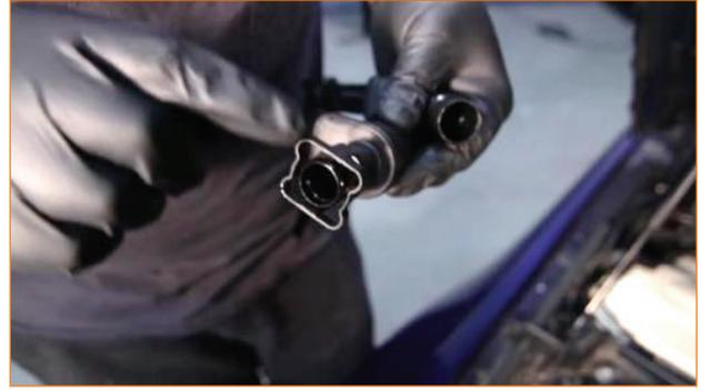
16. Reinstall the quick-disconnect fitting in its original location.
