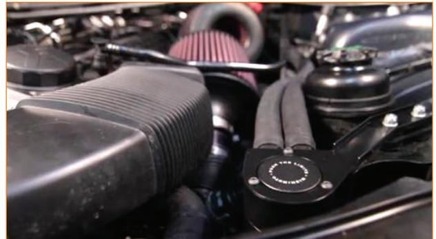
25. Reinstall the engine cover. (4x Allen bolts)
