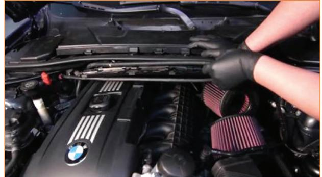
3. Remove the bottom half of the tray that holds the harnesses, and unfasten the three clips. (Pick tool or flathead screwdriver).
