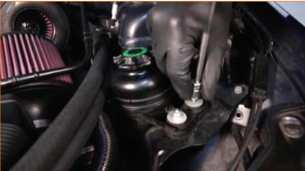
22. Using the two 10mm nuts removed in the previous step, install the catch can assembly onto the bracket and tighten the nuts.
