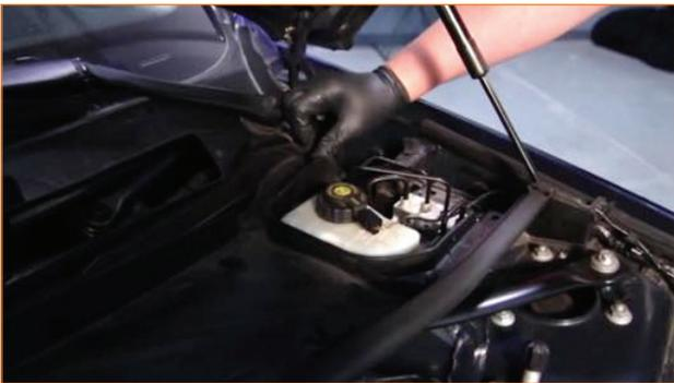
27. Reinstall the cabin filter using the coarse-threaded bolts that hold the filter to the main panel. (6x 8mm bolts)
