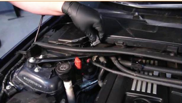
7. Remove the passenger-side panel by lifting up on the two side tabs and moving the last tab toward the cabin of the vehicle.
