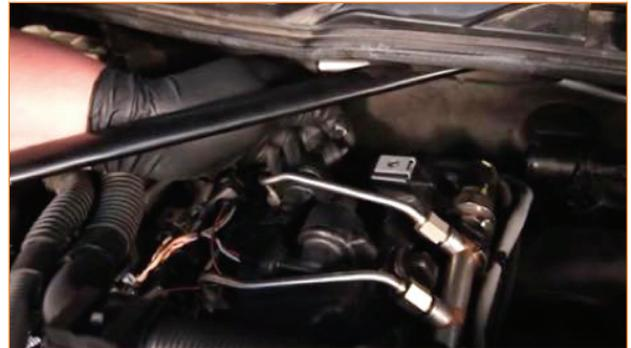
17. Take the first hose with the 180-degree bend, and slide it through so it seats properly. Attach this hose to the intake port, and then route the hose toward the front of the driver-side engine bay.
