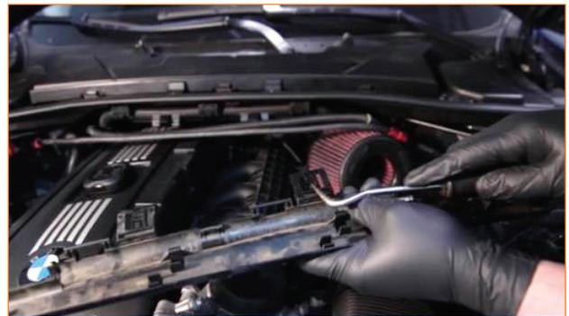
4. Remove the last wire harness. Unfasten the two clips and pull outward.
