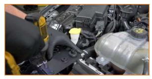
11. Connect the longer hose to the intake port on the engine and the outlet port on the catch can.(1x worm gear clamp)
