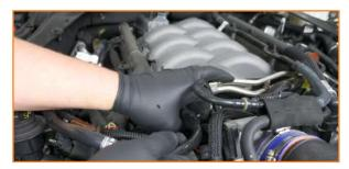
5. Remove the clips that secure the radiator cover. Once free, lift the radiator cover off the vehicle. (8x pop-clip)
