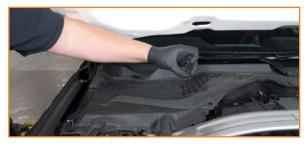
2. Remove the nuts that secure the strut brace on each side. (4x 15mm nuts)
