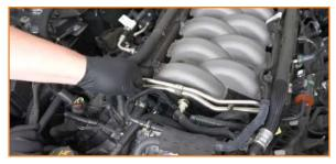
12. Connect the shorter hose to the PCV valve and inlet port on the catch can. (1x worm gear clamp)
