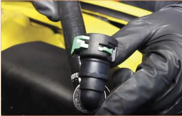
9. Route the shorter Mishimoto PCV hose so the end without a fitting is positioned near the driver-side strut tower; it should come up next to the intake manifold. Connect the fitting to the PCV valve, and lock down the quick-disconnect fitting by pushing the green tab into the fitting. Give the hose a gentle tug to make sure it is secured.
