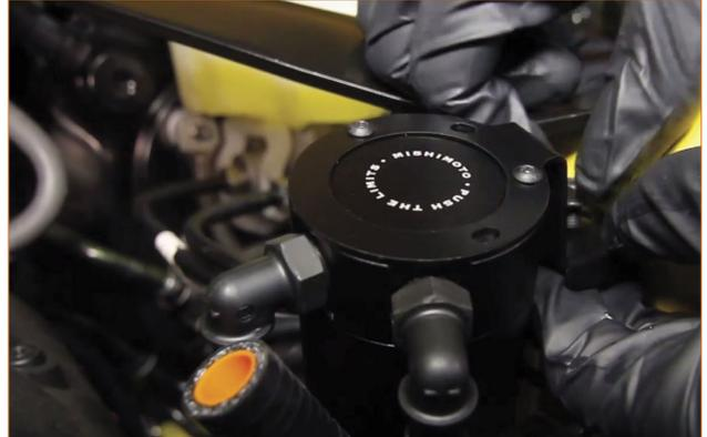
12. Slip two worm-gear clamps onto the Mishimoto hoses. (2x worm-gear clamps)
