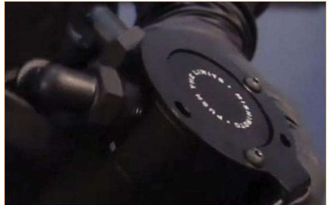
3. Install the supplied fittings on the catch can, ensuring that the elbows face downward (away from the bracket) before tightening completely. These fittings have tapered threads and do not need to bottom out in the catch can to seal properly.
