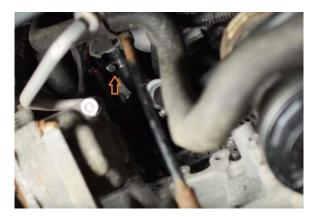
11. Tighten the clamps at all connections.
