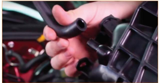
27. Connect the 90-degree hose to the intake manifold port. Route the hose so that the free end will sit just in front of the brake master cylinder when the manifold is installed.
