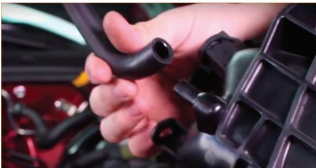
4. Detach the PCV hose from the purple nipple on the engine and from the PCV port on the back of the intake manifold. Remove the hose from the engine bay and set aside.
