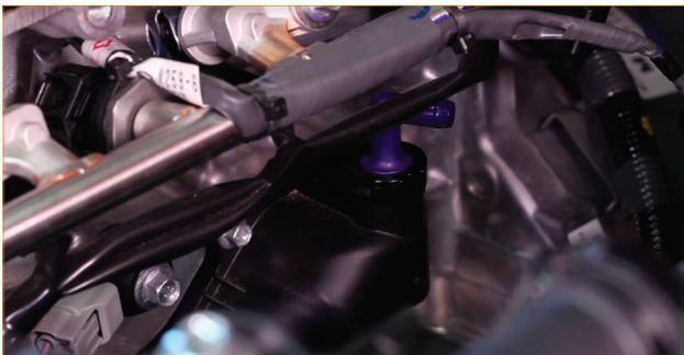
3. Reach around the back of the intake manifold (the firewall side) and locate the PCV hose where it attaches to the purple nipple on the PCV vent assembly (on the side of the engine block). The PCV hose is a short, U-shaped hose with no clamps.
