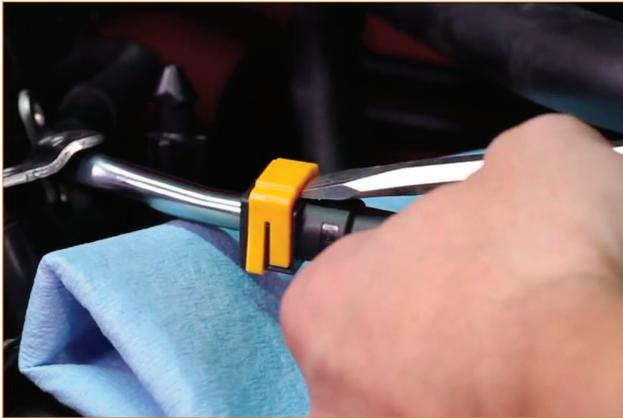
15. Clean up all the spilled fuel, and dispose of the rag properly.
