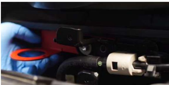
9. Place the fuel line back into the two clips. Make sure the top clip locks.
