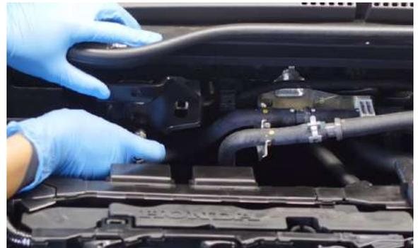
5. Release the fuel line from the two clips holding it in place. For the top one, use a flathead screwdriver to press in on the tabs clip before pulling it open.
