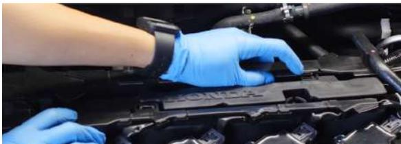
3. Compress the clamps on the ends of the PCV hose to separate them from their respective ports. Then, remove the PCV hose from the engine. (2x spring clamps)
