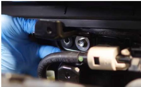
8. Install the Mishimoto catch can bracket behind the fuel line bracket and secure it with the original two bolts. (2x 10mm bolts)
