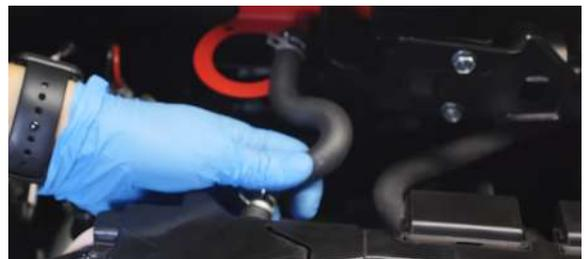
14. Install the catch can to the bracket using the hardware included in your kit. (2x 2.5mm screws)
