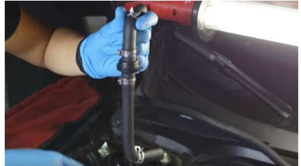
12. Install the unmarked end of the hose with a check-valve to the intake manifold.
