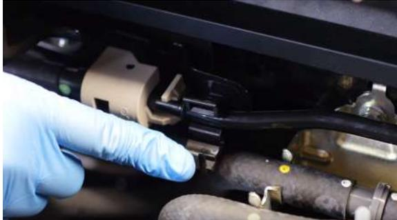
6. Carefully lean the rigid fuel line away from the clips to gain access to two bolts behind it.
