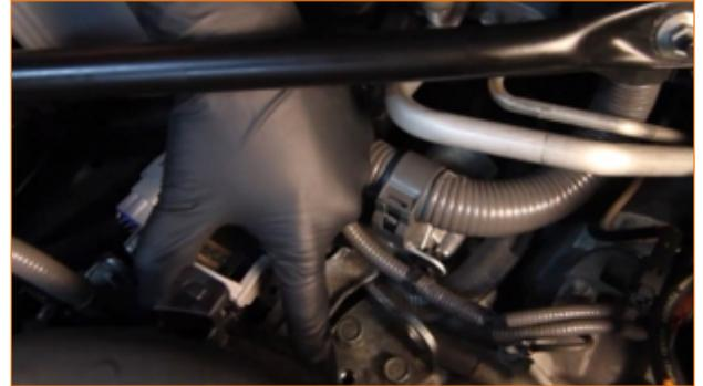
4. Remove the 1x 12mm nut from the driver-side shock-tower brace.
