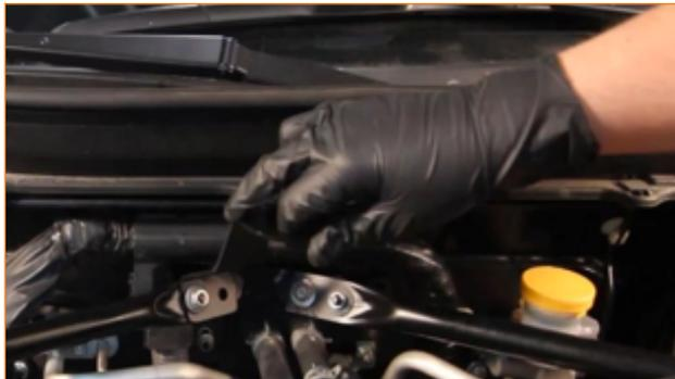
7. Reinstall the 1x 12mm nut that was removed from the driver-side shock-tower brace.
