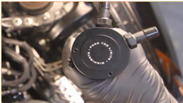
10. You can now tighten the fittings onto the catch can. [18mm socket]
