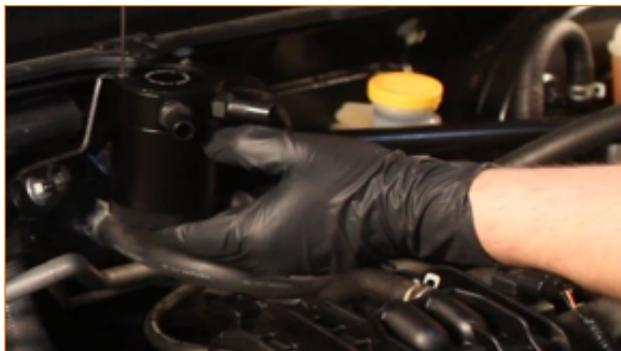
12. Install the silicone hose that runs from the in port on the catch can to the PCV valve. [2x worm-gear clamps]
