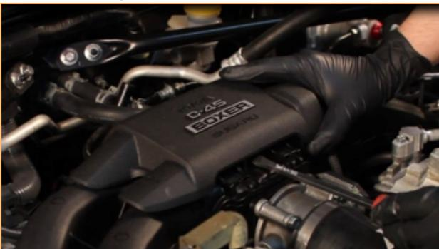
2. Remove the driver-side hose on top of the intake manifold. (Note: This hose does not have a clamp.)
