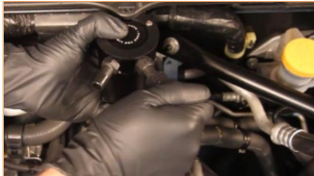
13. Install the silicone hose that runs from the out port on the catch can to the intake manifold. [2x worm-gear clamps]
