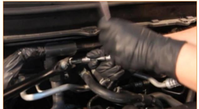
5. Loosen the remaining engine-side 1x 12mm nut from the driver-side shock-tower brace.
