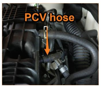
**07.** Route the MM4547-03 under the passenger side intake tube and connect it to the PCV valve located on the valve cover using 1x provided worm gear clamp. [1x MM1325-2]
