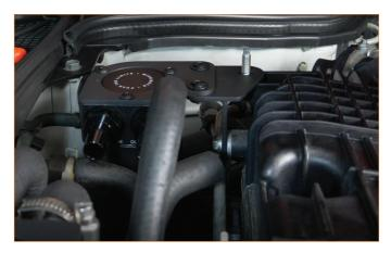
17. Connect the MM4547-03 hose to the port labeled "IN" on the MM1570 catch can using 1x provided worm gear clamp. Connect the MM4547-04 hose to the port labeled "OUT" on the MM1570 catch can using 1x provided worm gear clamp. [2x MM1325-3]
