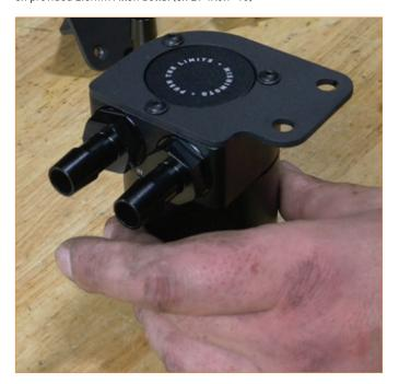
11. Fasten the MM2361-01 bracket to the MM1720 catch can using 3x provided 2.5mm Allen bolts. (3x BF4X0.7-10)
