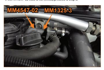
**05.** Remove the driver-side CCV resonator and replace it with the provided t-fitting, hose, and worm gear clamps as shown in the image above. (1x MM1410-01, 1x MM1410-02, and 3x MM1325-3)
