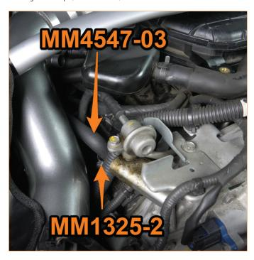
**08.** Connect the MM4547-04 to the port on the back of the intake manifold using 1x provided worm gear clamp. (1x MM1325-2)
