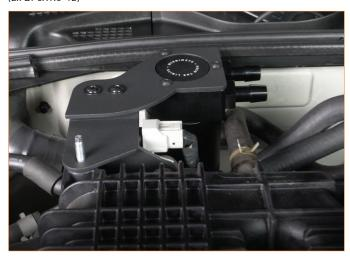
**14.** Connect the MM4547-02 hose to the port labeled **"OUT"** on the MM1720 catch can using 1x provided worm gear clamp. Connect the MM4547-01 hose to the port labeled **"IN"** on the MM1720 catch can using 1x provided worm gear clamp. [2x MM1325-3]
