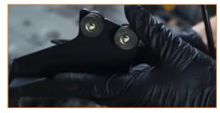
Install the Mishimoto catch can bracket using the original hardware from the stock bracket. Make sure to attach the power steering fluid container to the available slot on the Mishimoto bracket. (2x 10mm bolts)
