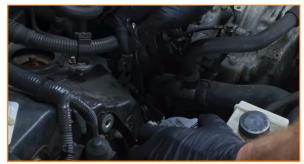
2. Slide the clamps down the hose connected to the PCV system. This will allow you to separate the hose from the valve cover and intake manifold ports. (2x spring clamps)
