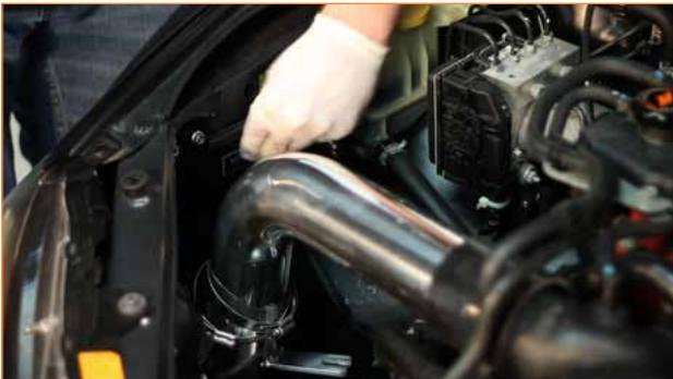
**7.** Using the two 10mm nuts that were removed from the factory airbox bracket, loosely secure the heat shield to the mounting studs in the engine bay.
