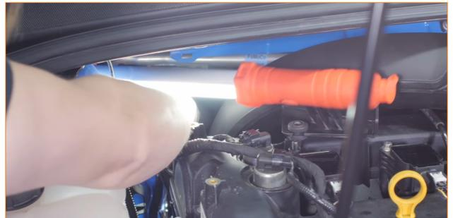
15. Separate the upper intake tube from the turbocharger, lift it off the mounting studs and rotate it to access the hose connected to the back of the tube. Disconnect this hose by squeezing the knurled tabs.
