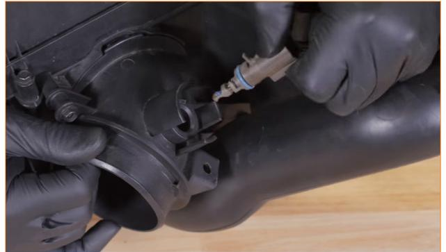
24. Remove the air inlet ducts from the stock airbox.
