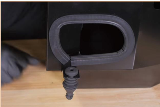
23. Remove the sensor from the stock airbox. Lift the lock tab on the sensor and turn the sensor counterclockwise by 90° to release it. Then pull the sensor straight out.
