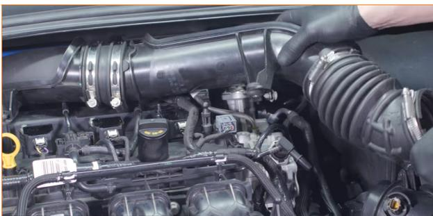
13. Separate the airbox from the vehicle by lifting it upward. The airbox is held in with three studs and grommets.
