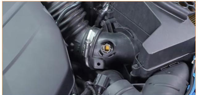
09. Remove the engine cover by lifting it directly upward. The cover is held in by four pegs and grommets.
