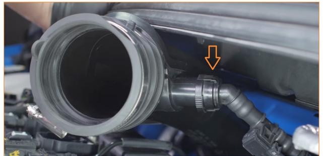
16. Remove the upper intake tube from the vehicle. Rotate the tube as you lift it out for easy clearance.
