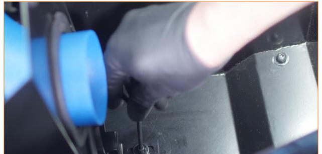
35. Secure the vacuum line to the induction pipe and reconnect the pipe to the vacuum pump.
