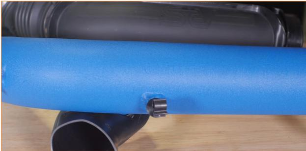
29. Remove the metal insert and rubber grommet from the stock intake tube. Transfer the insert and grommet to the bracket included with your kit. Then install the bracket to the Mishimoto induction pipe with the included bolt as shown here. Leave the bolt loose for now. (1x 10mm bolt)
