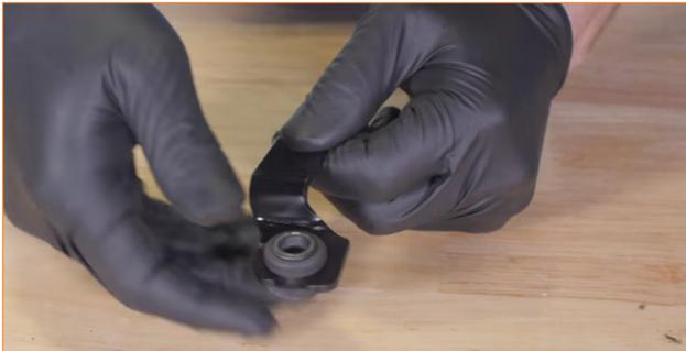
30. Remove the remaining metal inserts and grommets from the stock intake tube and transfer them to the last bracket in your kit. Set this bracket aside for now.
