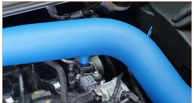
33. Install the air inlet duct to the airbox. Push the airbox down to engage the mounting pegs, and secure the air inlet ducts with the rubber shrouding.
