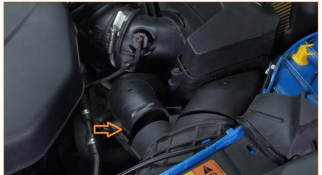
08. Separate the tree clip that secures the harness to the airbox, and disconnect the harness from the sensor.
