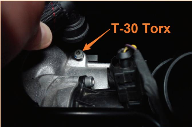
**4.** Rotate the stock turbo inlet pipe clockwise (towards the firewall) and then pull it away from the turbocharger to remove.
