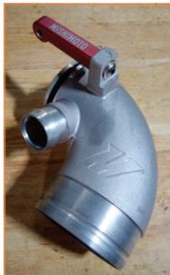
**6.** Align the Mishimoto turbo inlet pipe with the turbocharger inlet, then push inward and rotate counterclockwise. Tighten the T-30 Torx bolt first, then tighten the Allen bolt.
