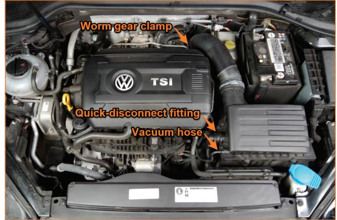
**2.** Remove the stock airbox and intake tube. (1x worm gear clamp, 1x vacuum hose, 1x quick-disconnect fitting)
