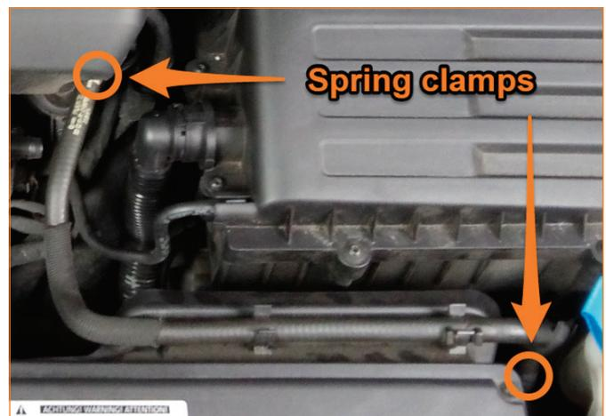
**4.** Remove the stock coolant hose from the driver's side of the radiator. (2x spring clamps)
