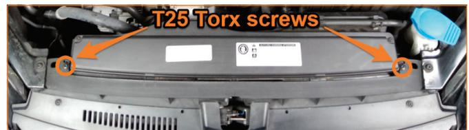
**3.** Remove the stock air duct. (2x T25 torx screws)
