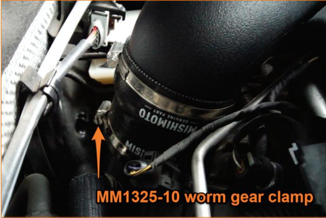
**11.** Secure the coupler to the turbo inlet pipe using the provided worm gear clamp. (1x MM1325-10)
