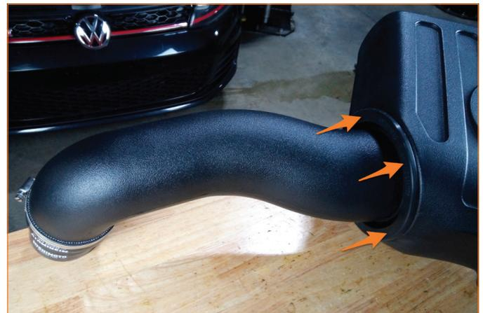
**9.** Install the intake tube assembly into the airbox. Starting from one spot, push the intake tube grommet into the airbox cutout until it is fully seated.
