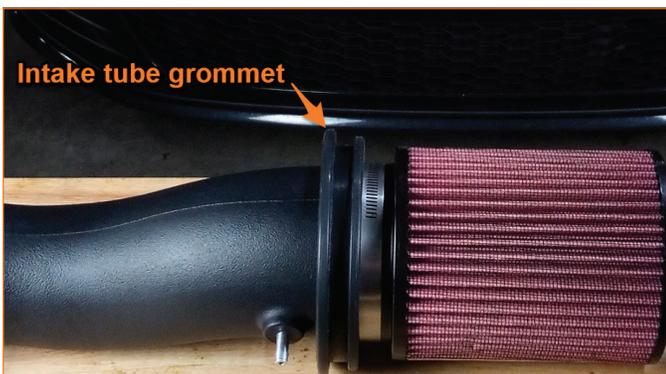
**7.** Slide the intake tube grommet over the intake tube, then install the air filter. (1x MM4545, 1x MM1672)
