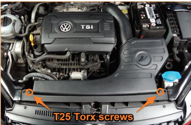
**13.** Secure the front of the airbox to the vehicle using the 2x T25 torx screws removed in step 2.
