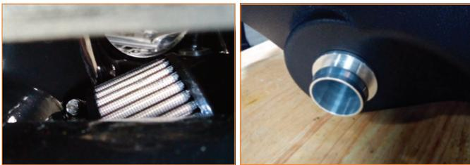
**6.** Install the secondary air injection system filter into the Mishimoto airbox. (1x MM79-09, 1x MM1700-01)
