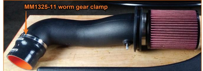
**8.** Install the coupler to the intake tube using the provided worm gear clamp. (1x MM1325-11)
