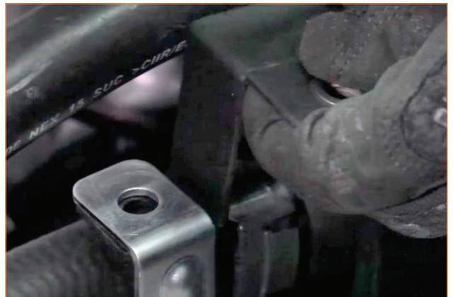
17. Install the coupler over the throttle body, and slip two worm-gear clamps over the coupler. Orient the clamps so that the adjustment nut will be accessible. Then tighten the clamp that secures the coupler to the throttle body. (2x worm-gear clamps)
