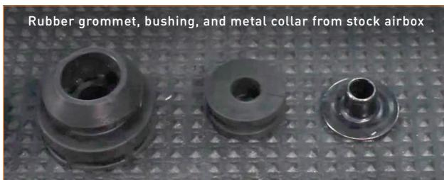
Rubber grommet, bushing, and metal collar from stock airbox
