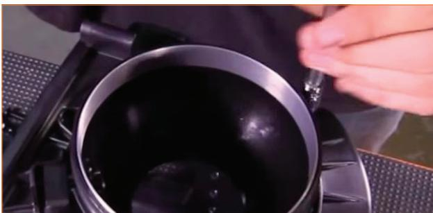
18. Release the MAP sensor from the adaptor by turning it counterclockwise, and then remove the sensor.
