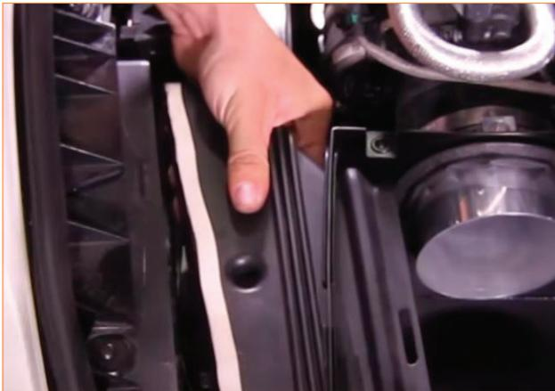
26. Install the air filter to the intake pipe and secure it with the worm-gear clamp.
