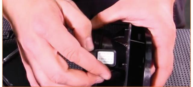
19. Install the stock airbox mounting bracket onto the Mishimoto airbox. Orient the bracket so the dowels point downward, in the same direction as the dowel on the airbox. The 7mm bolts install from inside the box, through the smaller holes. The 10mm bolts install from outside the box, through the larger holes. Orient the bracket so it is flush with the side of the box before fully tightening the bolts. (2x 7mm nuts and bolts, 2x 10mm nuts and bolts)
