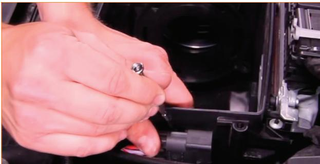
10. Disconnect the electrical harnesses from the ECU. Each connector is secured by a lock lever. Depress the black tab that holds the lock lever, and then lift the lever to release the connector. Disconnect both harnesses, and set them out of the way.
