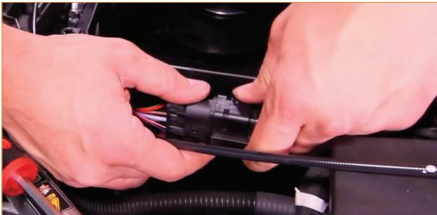
09. Remove the female end of this connector from the airbox. To release the connector, slide a small screwdriver between the connector and the airbox to depress the locking tab. Then slide the connector down and off the airbox.
