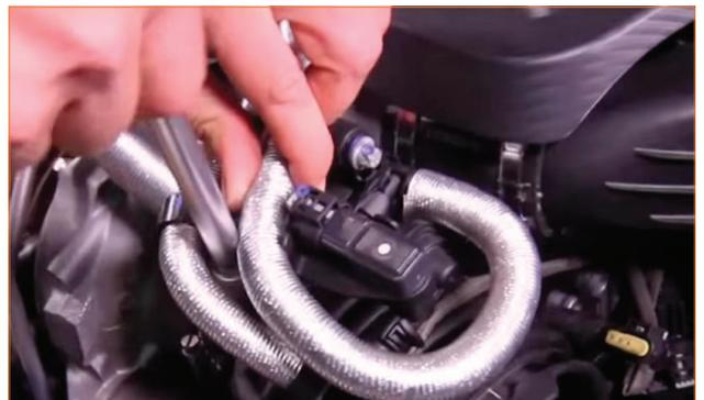
13. Remove the bracket that held the PCV/boost solenoid assembly you just removed. Remove the bolt that secures it, and then wiggle the bracket to aid in removal. (1x T45 Torx bolt)
