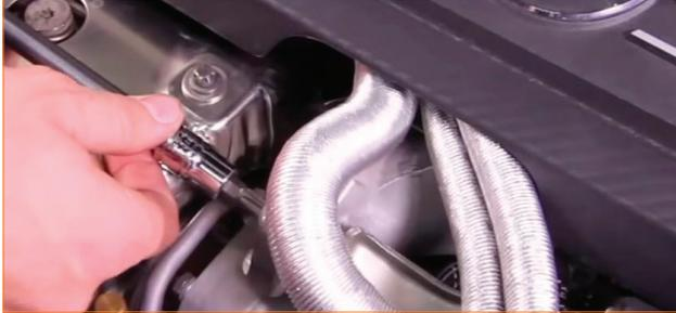
14. Loosen the worm-gear clamp that connects the intake boot to the turbo, and then remove the intake boot.
