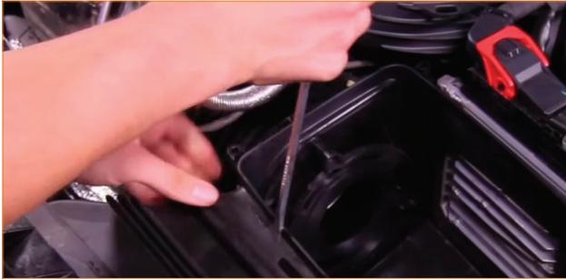
08. Separate the wiring harness connector on the side of the airbox. Push the gray tab out of the connector and then depress the tab to release the connector.
