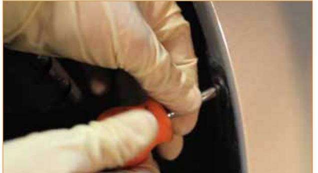
7. Remove both side marker housings. After pulling out the housing, locate the clip on the inside of the marker housing slot. Remove this clip on both the driver and passenger sides of the bumper.
