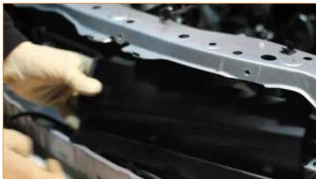
3. Remove the six 12mm bolts for the upper radiator support. Two of these bolts are located on the lower portion of the support between the electric fans. Do not remove the radiator support unit completely.
