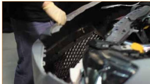
**2.** To make the installation of the side marker assembly easier, route the harness through the slot in the bumper for both the driver and passenger sides.
