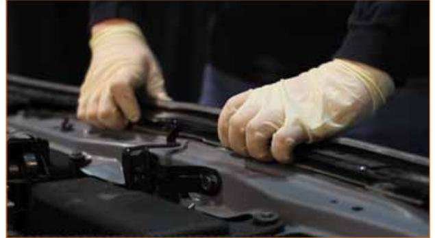
6. Remove the three small fender clips located in both the passenger and driver side fender wells.
