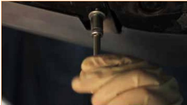
11. Now that all the bumper hardware has been removed, the bumper can be separated from the vehicle. Carefully pull the bumper away from the vehicle; an audible pop will be heard as the bumper unclips.
