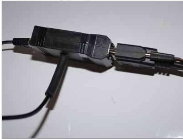
**12** Connect the vacuum line and harness to the control box as shown. (note: for versions earlier than 2.1, the vacuum port is on the harness)
