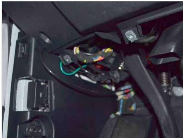
**14** Replace the side kick panel and tuck/secure the control box and harness up above this panel near the other factory wiring.
