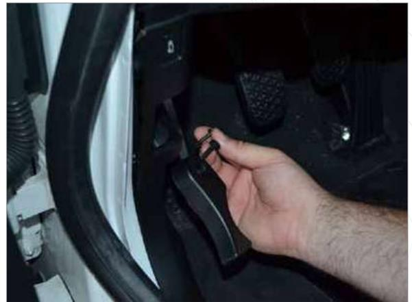
**15** Replace the hood pop lever and then replace the footwell cover below the steering wheel.
