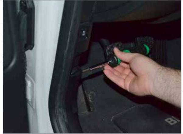
**7** Remove the side kick panel cover screws, first remove the Phillips screw holding the hood pop lever, then the screw behind the lever. 2 screws total.
