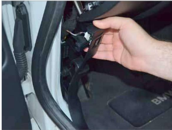
**8** Flex this panel forward to get access to the OBD2 port and the trunk pop switch. You will need to pull the rubber door seal forward to free the panel.
