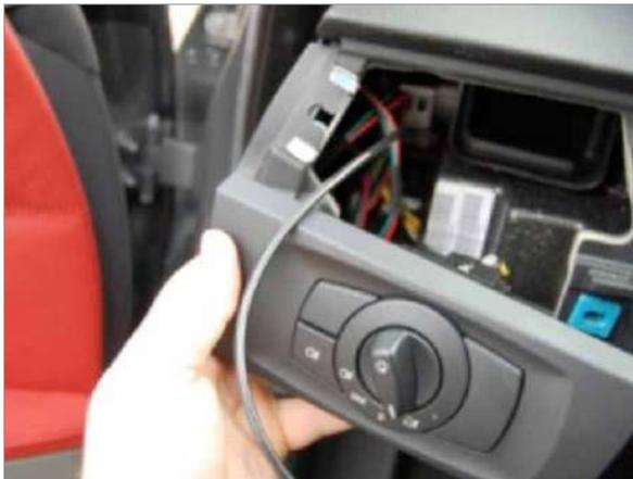
**5** Remove the light switch assembly to give yourself room to work, it just pulls out.
