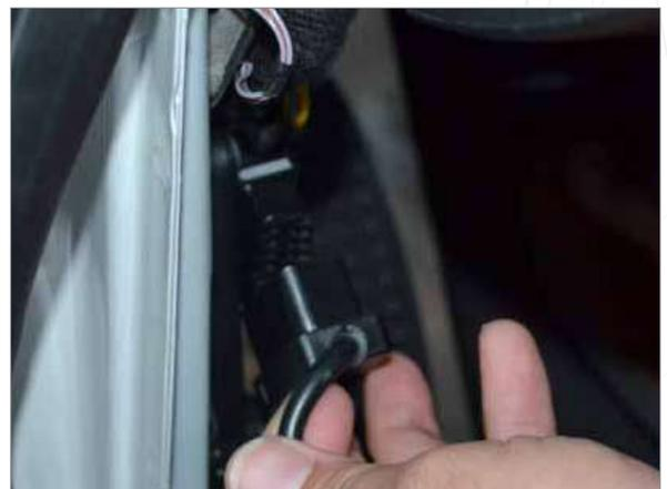
**11** Plug in the obd2 connector to the car.
