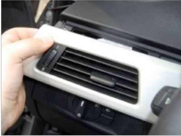
**1** With the driver's door open, remove the vent from the car with trim attached. Pull straight out or use a cloth covered screwdriver on the outside of the vent trim. The vent and trim come out as one piece.
