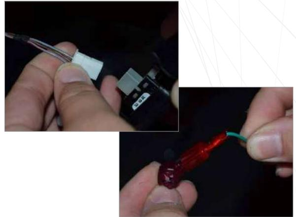
**9** (Optional) To use the auto dimmer, D.On.A function of the gauge, connect the GREEN harness wire to the Red/Gray wire on the TRUNK POP SWITCH with the T-Tap connector. If you do not tap this wire for dimmer, you can use the one-touch manual dimmer option on the gauge.
