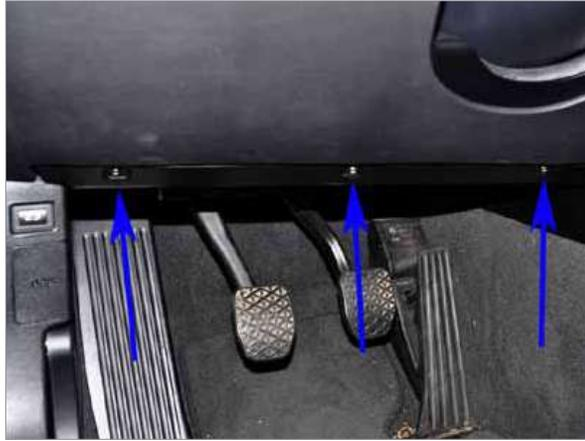
**6** Remove the lower dash cover below the steering wheel by removing the three #20 torx screws shown here. Lay this cover down into the footwell.
