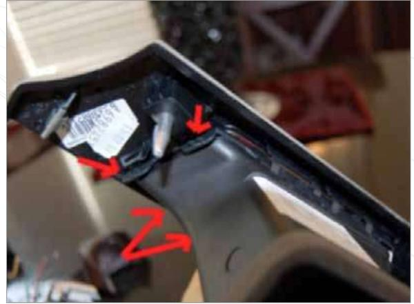
**2** Unclip the vent from the trim; release it from the clips on one side and bottom, then pull away to release the other side.
