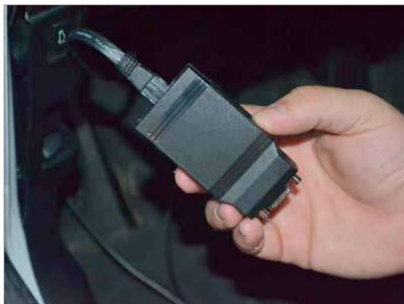
**10** Feed the display wire down to the lower dash footwell area and connect it to the control box.
