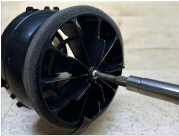
**7** Tighten screw until head touches vent housing (do not over tighten)
