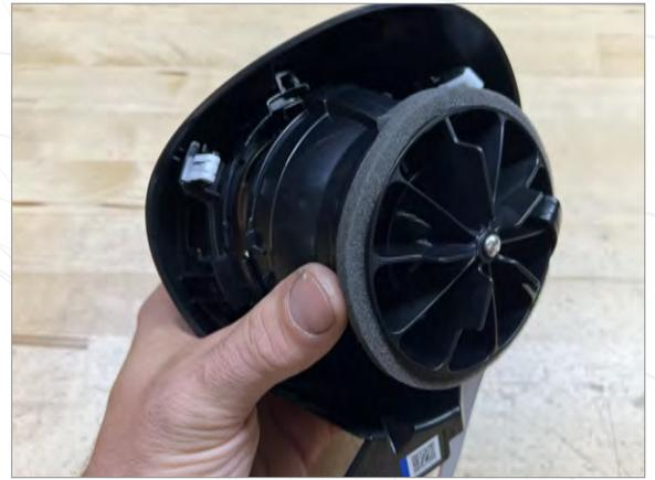
**8** Snap the trim back onto the vent housing making sure to line up the notch at the top of each part
