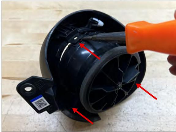
**1** Use a screwdriver or pry tool to disconnect the 3 clips on the vent trim and then remove vent trim from housing
