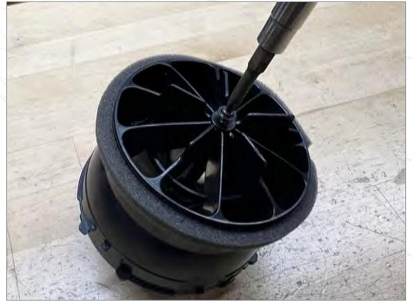
**2** Remove screw from back of vent housing
