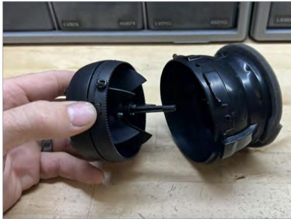
**3** Remove internal mechanism from vent housing
