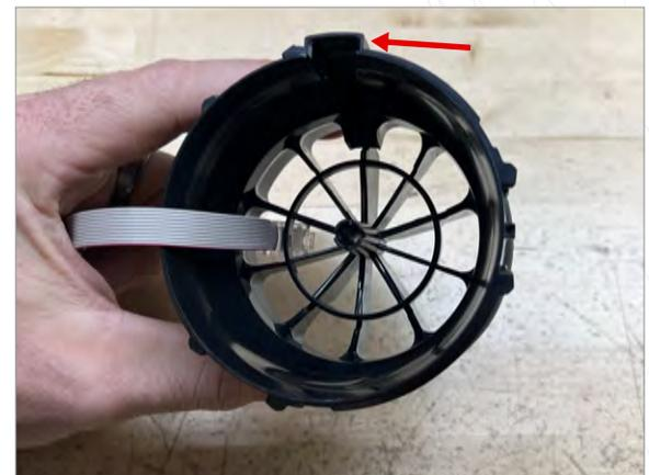
**4** Insert display ribbon cable as shown. Note the orientation of the notch in the vent (12 O'Clock Position)
