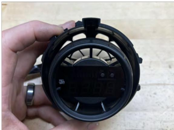
**5** Install the display into the vent housing as shown, making sure the notch is at the top of the display
