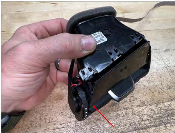
**7b** Snap display pegs into place on left side
