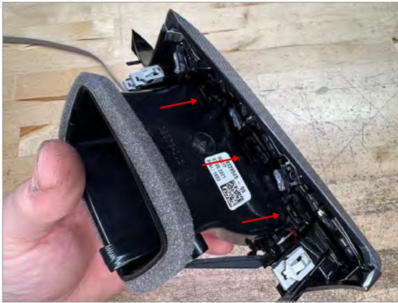
**9a** Reinstall trim by snapping 3 clips on top into place
