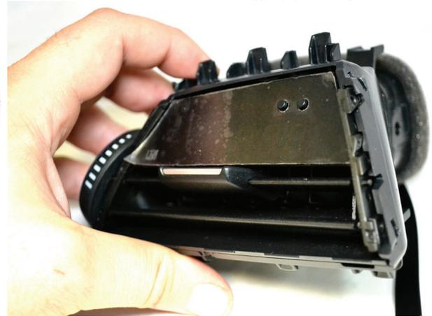
**6** Make sure the VIDI display tabs are in the holes, and then press the entire assembly fully into the vent housing.
