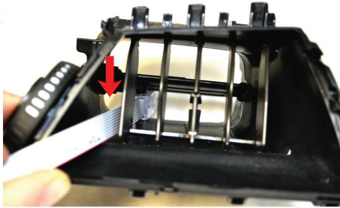
**4** Insert the VIDI Display cable through the FAR LEFT side of the vent and out the back UNDER the open/close flap. Feed all the slack through.
