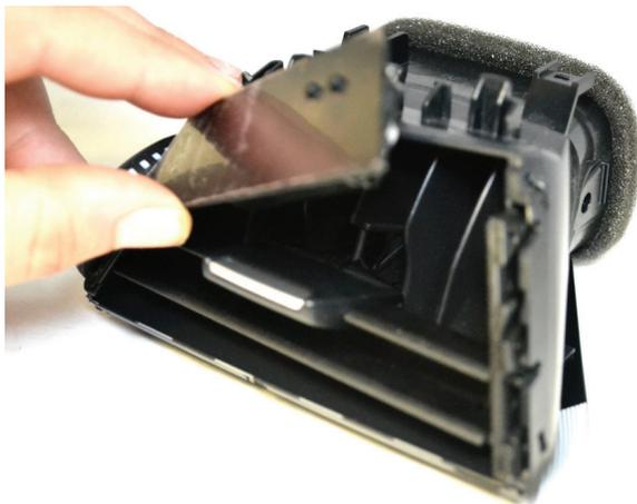
**5** Replace the bottom slats and the vent slat holder on the far side, and insert the P3 VIDI display into the upper 4 holes where the 2 top slats were removed.
