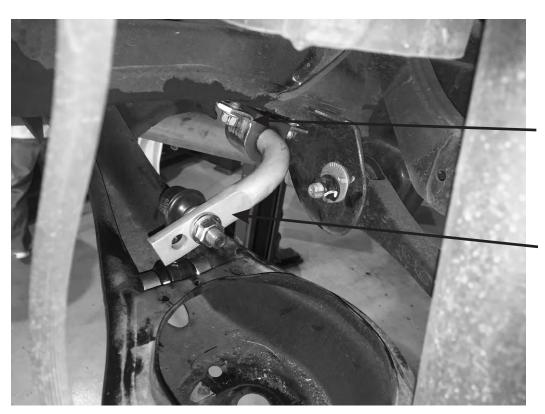
Loosen swaybar saddle to help with install of links
