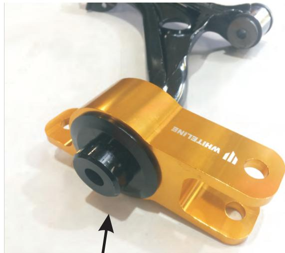
• Steel arm and bushing insert **69192** shown
