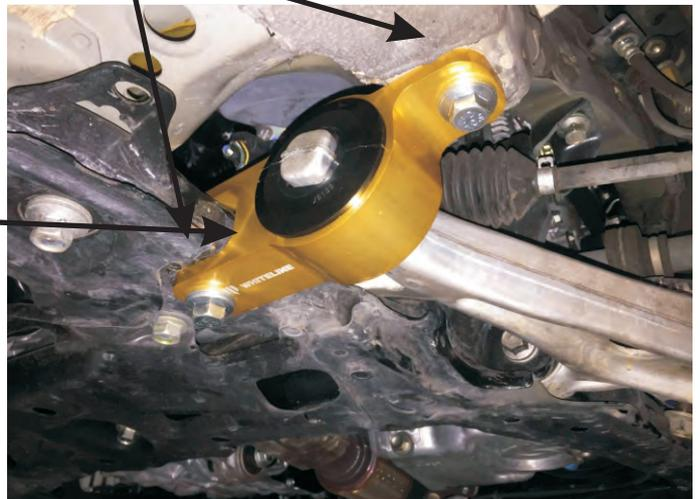
• Aluminium arm and bushing insert **69156** shown
