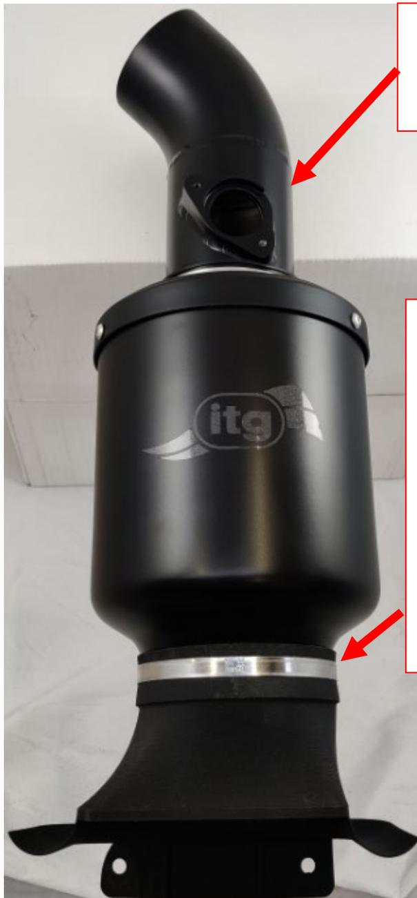
Insert MAF Tube into Rubber Grommet in Filter lid.
