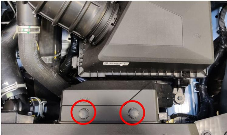
Prize upwards as shown, with a small flathead screwdriver or trim removal tool.
