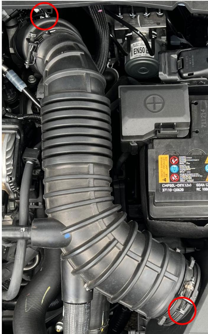
3) Pull the hose off the turbo & the airbox lid – remove from the car.
