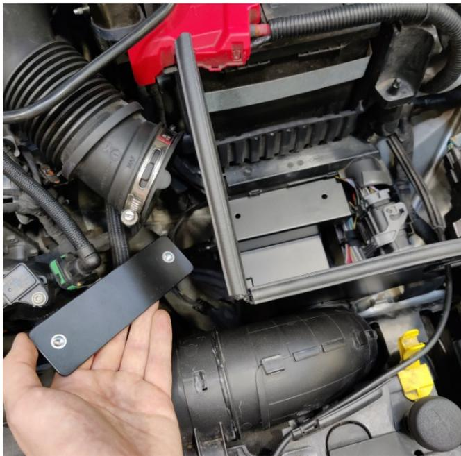
**Note:** The two holes in the lower bracket are offset. To fit this bracket, it must be orientated with the shortest gap from the edge pointing towards the rear of the car (as shown)
