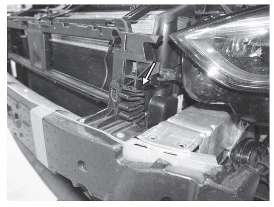
57) Place the crash beam back on the car, ensuring the accordian part from crash beam connects into the tabs of the upper bumper support.
