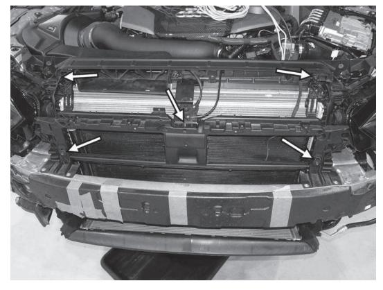
61) After realigning the upper bumper support, tighten all five T30 screws to 5Nm (44in-lbs).
