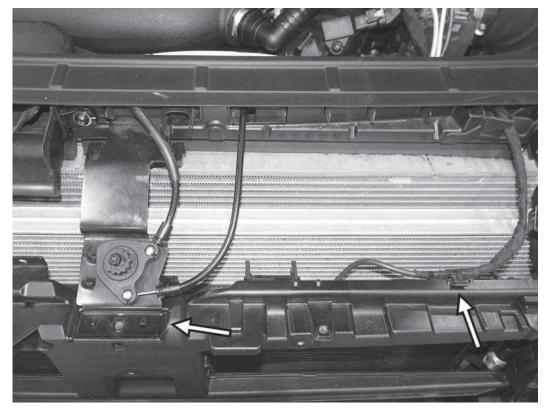
19) Separate the hood latch mounting bracket from the upper bumper support. Remove the clip holding the front camera wiring harness to the upper bumper support.
