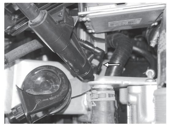
21) Disconnect the washer fluid line from behind the back of the left headlight washer by pressing on the blue tab. Also disconnect the washer line that is on the right side of the bumper crash beam. The washer line will stay attached to the crash beam.
