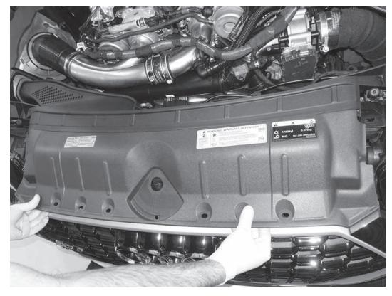
73) Place the upper bumper cover back on the car. Place the back side of the cover into the radiator core support, and then lower the front side of the cover behind the front grille.
