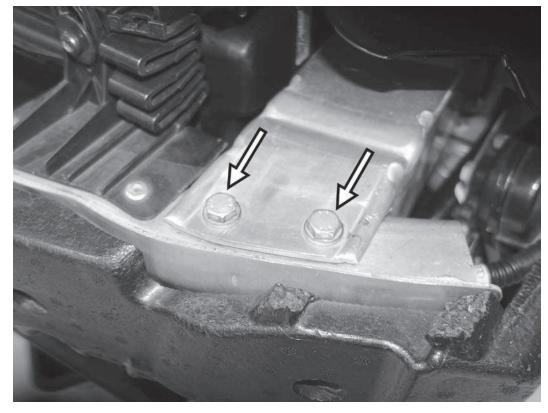
59) Push the bumper crash beam back in place. A deadblow hammer may be needed to push the crash beam back to its original mounting points. Install the four 13mm screws and nuts holding the crash beam in place, and tighten them to 23Nm (17ft-lbs).
