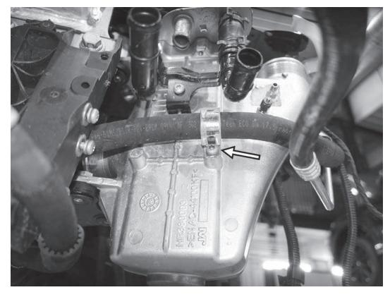
35) Remove the T30 screw holding the air conditioning line from the front of the stock intercooler. Remove the bracket from the AC line as well.
