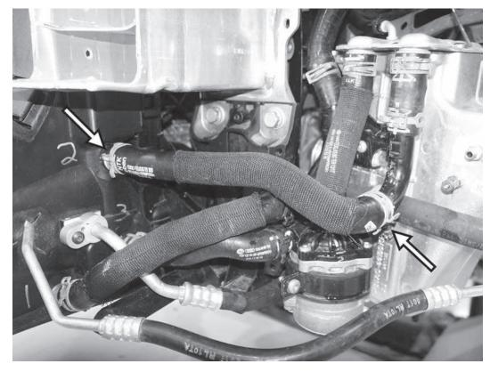
29) Loosen the two spring clamps on the coolant hose on the top of the auxillary radiator, and remove the hose from the car. Be aware coolant will spill as these hoses are removed.
