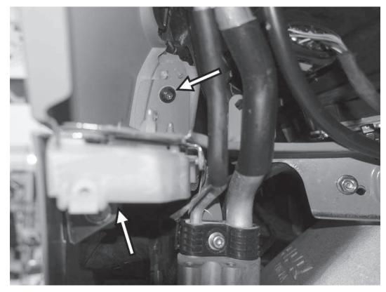
71) Reinstall the T30 screws holding the bumper cover to the front side of the fender. Install the push pin style connectors that go between the side of the bumper cover and the bottom of the front fenders.
