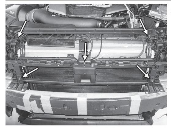
17) Remove the five T30 screws holding the upper bumper support to the radiator core support.
