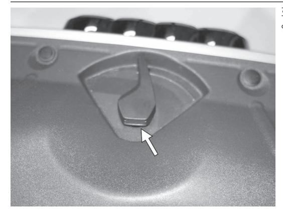
75) Reinstall the hood release latch. The latch is keyed, so it can only go on in one position.
