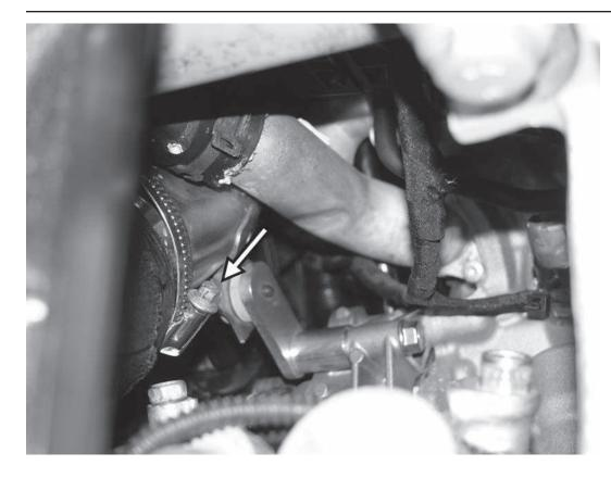
27) Loosen the 7mm hose clamp holding the lower intercooler hose to the factory metal charge pipe.
