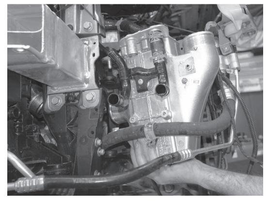
37) Lift up on the stock intercooler to remove it from the stock mounting bracket. Remove the stock intercooler from the car.
