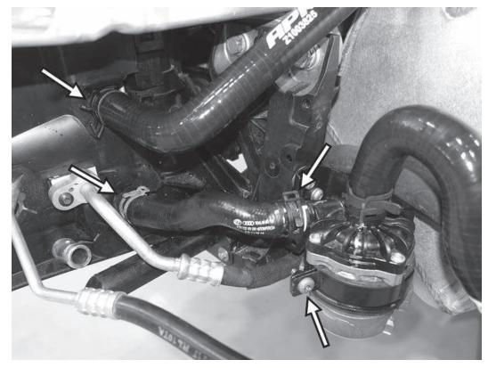
49) Reconnect the factory coolant hose to the side of the coolant pump, and then to the connection by the radiator support and secure with the spring clamps. Connect the other end of the previously installed APR hose (Z1003825) to the top connection of the front radiator and secure with a spring clamp. Finally, when the factory coolant hose is without tension, fully tighten the T30 screw on the coolant pump bracket to 9Nm (80in-lbs).
