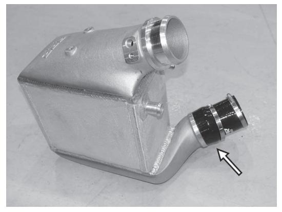
39) Install the APR lower intercooler hose (Z1003822) loosely onto the inlet of the APR intercooler. Loosely secure the hose with the supplied hose clamp.
