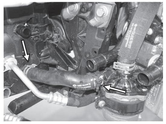
31) Loosen the two spring clamps on the coolant hose going into the side of the auxillary coolant pump, and remove the hose from the car.
