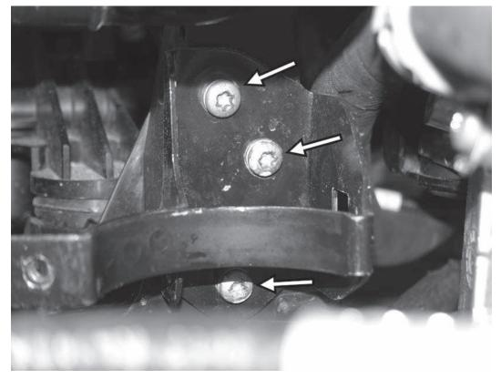
33) Remove the three T30 screws holding the auxillary coolant pump bracket to the side of the radiator support, and remove the bracket from the car.
