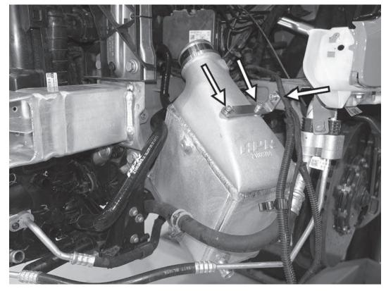
41) Place the APR intercooler in the car where the stock intercooler and stock bracket were. Loosely connect the lower intercooler hose as you place the intercooler. Loosely attach the upper APR mounting bracket to the intercooler with two of the supplied 5mm allen screws and flat washers. Use another 5mm allen screw and flat washer with the supplied 10mm flanged nut to attach the other side of the bracket to the slotted hole in the left fender support bracket.
