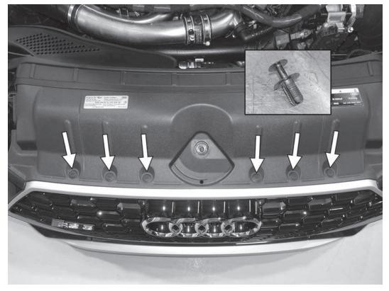
3) Remove the six push pin style connectors holding the cover between the front bumper and the radiator support. Carefully pry the raised center part of the pin up, and then remove the entire pin assembly up and out of the cover.
