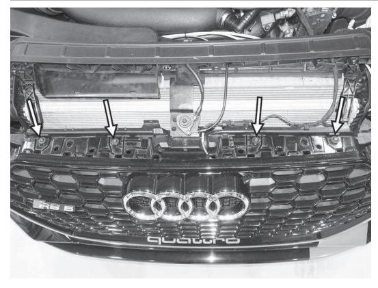
5) Remove the four T30 screws holding the top of the bumper cover to the upper bumper support.
