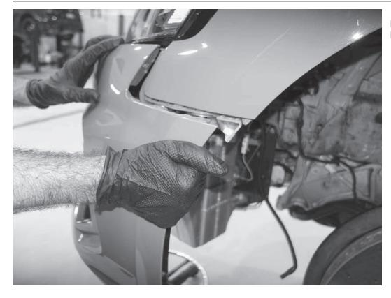
13) Carefully pull both sides of the bumper cover away from the bumper bracket on the bottom of the fender.
