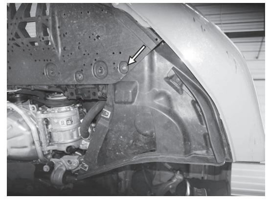
11) Remove the last T25 from both of the front wheel spoilers. Separate the headlight drain lines from the back of the spoilers, and then remove them from the car. The other fasteners to these spoilers should have been removed when uninstalling the wheel well liners.
