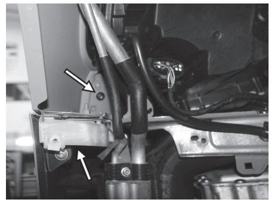
9) Remove the T30 screws holding the bumper cover to the front side of the fender. Also remove the push pin style connector between the side of the bumper cover and the bottom of the front fender. Repeat on the other side of the car.
