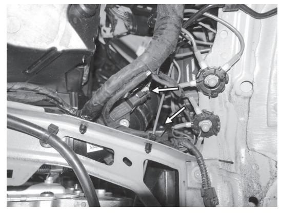
15) As seen from the front side of the left wheel well, disconnect the electrical connector to the MAP sensor that is on the throttle body inlet pipe assembly. Remove the 10mm nut that holds the bracket from the throttle body pipe to the left frame rail.
