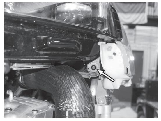
23) Remove the T30 screw from underneath the left headlight, by the front fender.
