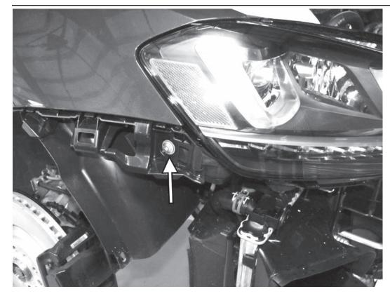
23) Remove the T30 screw from the side of both headlights.
