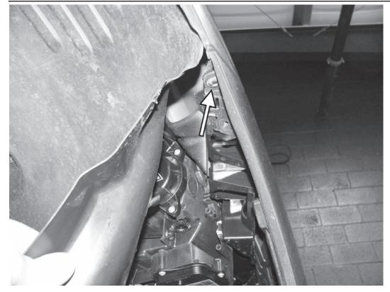
59) Pull back the fender liner, and install the one T25 screw that holds the corner of the bumper cover to the front fender. Repeat on the opposite side.
