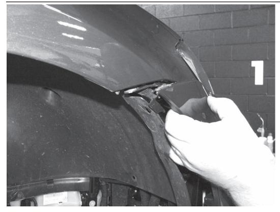
57) Pull the sides of the bumper cover back and snap into the mounting clips on both sides of the front fenders.
