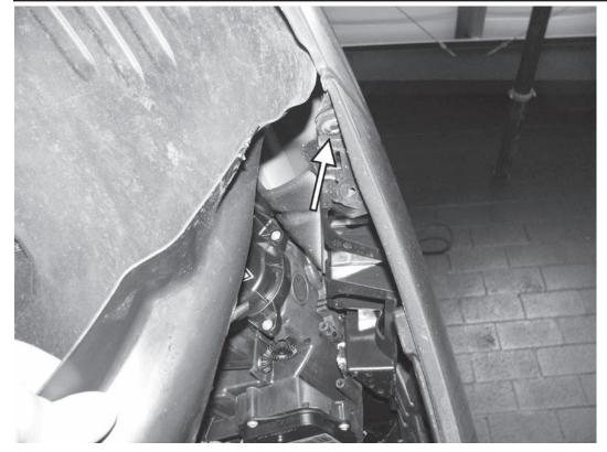
15) Pull back the fender liner, and remove the one T25 screw that holds the corner of the bumper cover to the front fender. Repeat on the opposite side.
