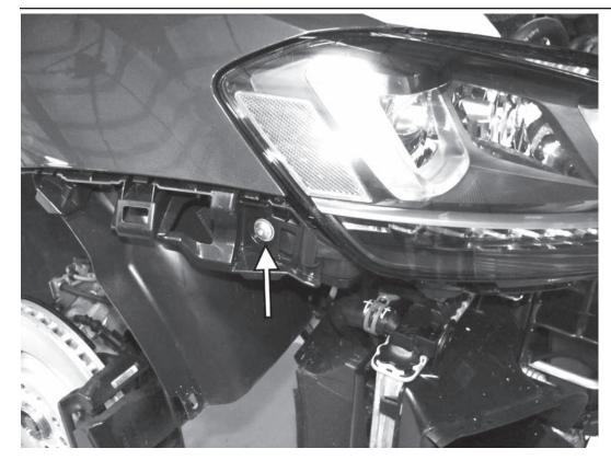
55) Reinstall the T30 screws on the outside of both headlights.
