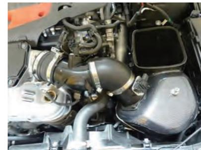
30. Connect the genuine suction pipe and air mass adapter with the included elbow hose and attach with a band. (Use attached hose band x2)
