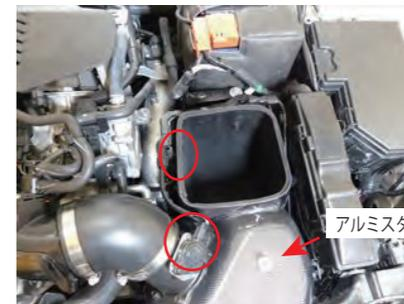
31. Attach the intermediate clamp of the air mass sensor to brace B. Then install the sensor coupler.
