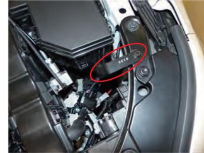
34. Place a rubber washer under brace B to secure it to the vehicle. (Using 1 bolt and 1 nut)
