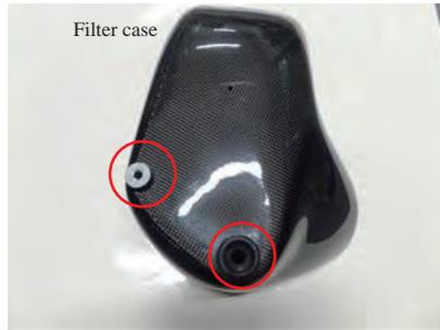
13. Attach the rubber bushing removed from the original filter box to the filter case.
