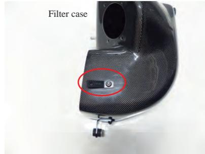
14. Attach brace B to the filter case. (Using 1 bolt A and 1 nut)
