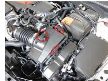
2. Remove the sensor wiring clasp and remove the wiring coupler.
