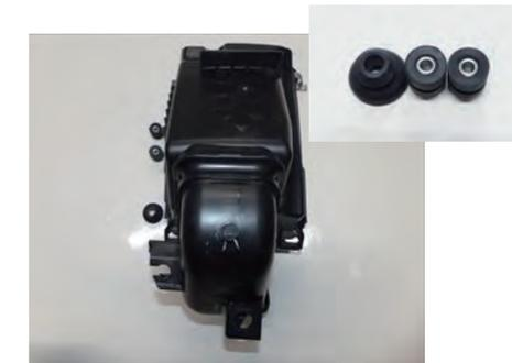
6. Remove the three rubber bushes from the bottom of the box.
