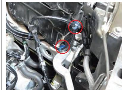
7. Unhook the sensor wiring.
