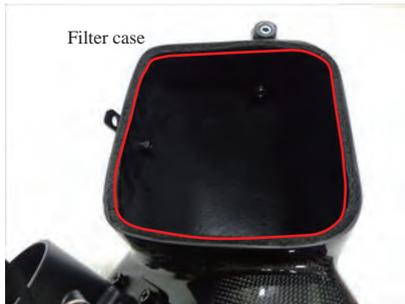
16. Apply sponge tape around the inside edge. (The rest of the cut will be used in step 23.)
