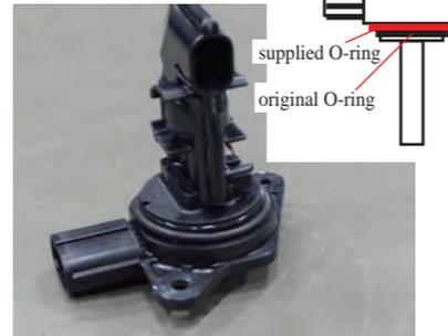
18. Attach the supplied O-ring to the air mass sensor by placing it on top of the original O-ring.
