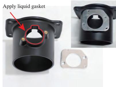
17. Apply the included liquid gasket to the arrow on the air mass adapter and install the conversion plate. (Using bolt F) Wipe off any spilled liquid.
