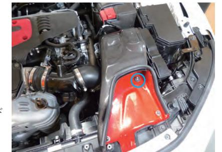
32. Place the introduction duct ASSY over the filter case and insert the rubber bushing into the aluminum stud.
