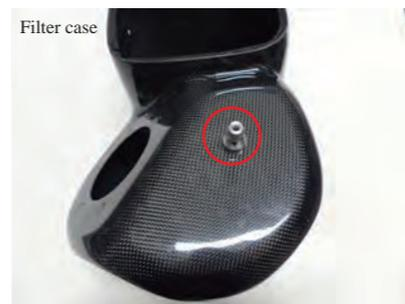
15. Attach the aluminum stud to the filter case. (Using Bolt Cx1)
