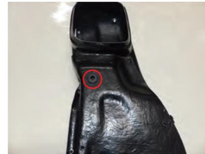
27. Attach the included rubber bushing to the introduction plate.
