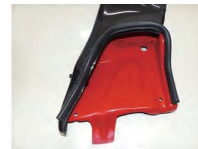
26. Attach the rubber molding removed from the original duct to the introduction duct ASSY. Insert the rubber molding pin and insert the lock ring on the back side to fasten it. (11 locations)
