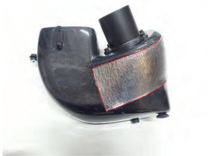
22. Attach the heat-resistant mat referring to the diagram above.
