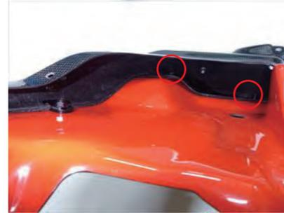
24. Assemble the introduction plate and introduction cover. Insert the bolt Ax2 from above and fix it with the nut x2.
