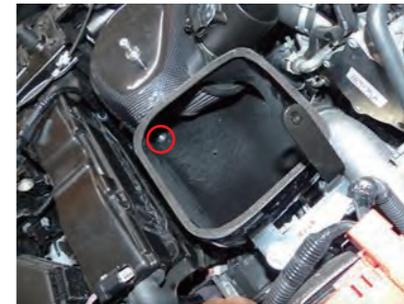
28. Place the carbon case ASSY on the vehicle. Fix the filter case with the original bolts.
