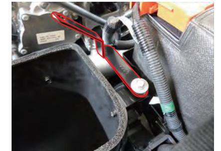
29. Fix brace E on top of brace A of the filter case using the original bolt.
