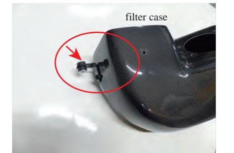
12. Attach the rubber bushing removed from the original filter box to brace A.
