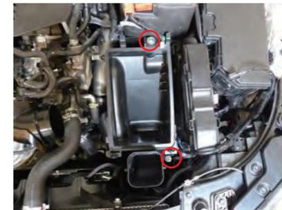
5. Remove the two bolts and remove the bottom of the box.
