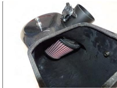
21. Put the filter in the filter case and tighten the band.
