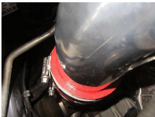
6. Apply a little lubricant inside the hose and fit the pipe to the car in the reverse order of removal.
