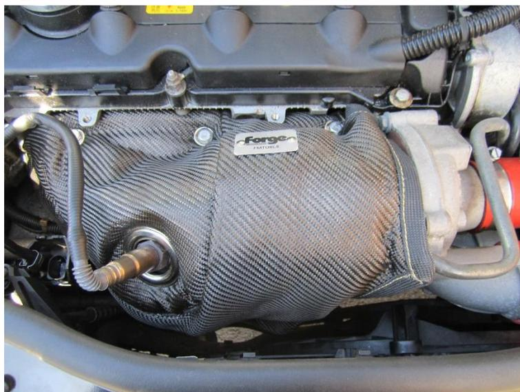
Please note that a turbo blanket will lose its flexibility over the first few heat cycles as the material cures, so once fitted it should **not** be routinely removed as this can cause damage to the blanket.
