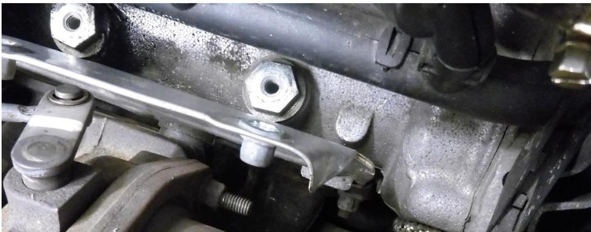
9. Depress the yellow locking clip and un-plug the lambda probe loom. Feed the lambda plug through the large hole on the FMTUBL16.
