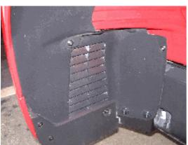
The vehicle was safely supported so that the front wheels could be removed. It was then necessary to remove the Hex screws that hold the wheel arch liner and the small lip spoiler in place.
