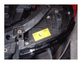
The head lights\* were removed by disconnecting the three plug connectors on the rear and removing the two top Hex bolts and the front Hex bolt
