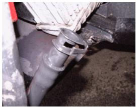
It was also necessary to disconnect the feed to the headlight washers. A small "U" clip allowed the hose to be separated. Prepare yourself with a suitable bucket or hose clamp before disconnecting as the entire reservoir will drain.
