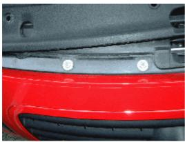
Next the bonnet landing panel plastic cover was removed by pressing the pins through the plastic clips. Then the bumper top mounting hex bolts were removed, although we left one in place until we were ready to lift the panel off, so that it didn't drop unexpectedly.
