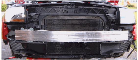
With the plastic front panel out of the way, the front alloy bumper was removed, it is held in place by 13mm nuts on "Allen" bolts. The two horns needed to be disconnected.
