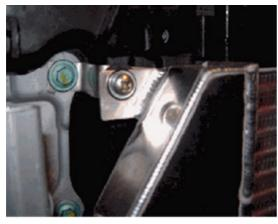
The intercooler mounting 6mm bolt was then passed through the rubber mounting into and secured in the captive nut on the angular bracket.
