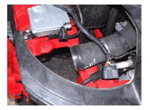
Next we needed to get ready for the new intercooler so we removed the 10mm bolt holding the ambient air temperature sensor in place. (sited on the lower front of the vehicle) and also the rubber mountings from the OEM intercoolers which need to be inserted into the 16mm holes on the Forge unit
