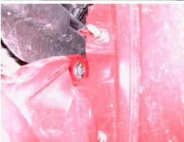
With the wheel arch liner out of the way the two 10mm nuts that hold the front panel to the wing were removed. Obviously these first two steps needed repeating on both sides of the vehicle.
