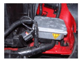
Also where the Xenon units are installed it is necessary to remove the right hand side transformer in order to gain access to the two 10mm bolts that are underneath and hold the intercooler bracket in place
