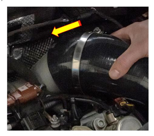
11. Using a 7mm ratchet and the remaining hose clamp attach the other end of the silicone hose to the air box. You can see in the images below where the silicone hose can be connected to either the OEM airbox or an induction kit (*in this case the Forge Motorsport FMINDK40*)
