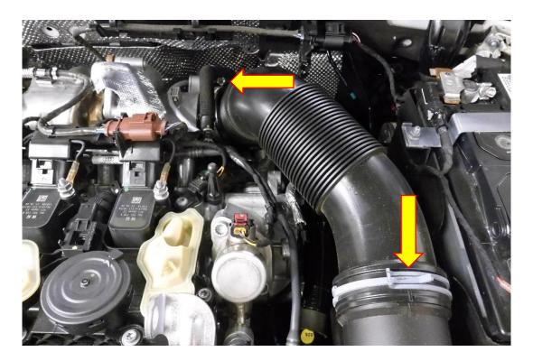
3. Depress both locking tabs on the breather hose and pull it away from the spout on the dump valve recirculating hose and then from the turbo adaptor.
