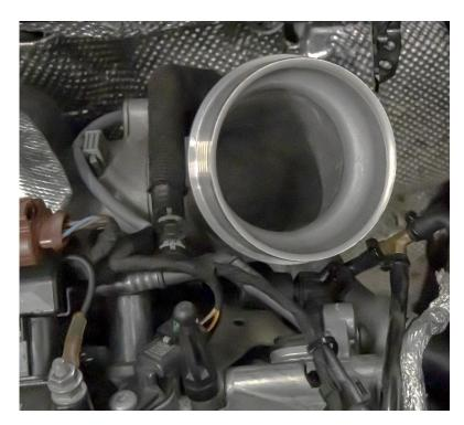
8. Push the breather hose into the machined breather adaptor that spouts off the side of *FMTIA9* till it clicks
