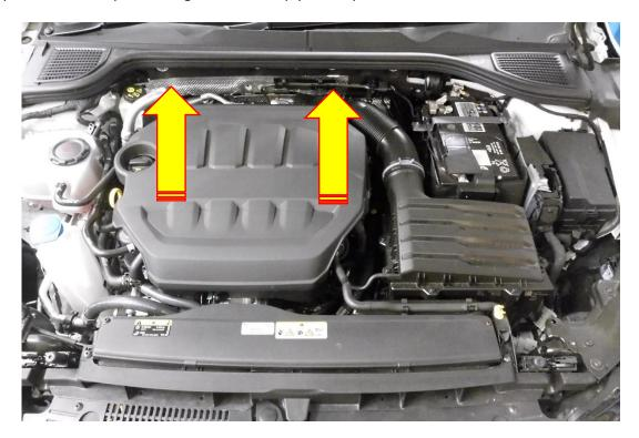
2. Using a hose clamp removal tool/long nose pliers and a 7mm socket and ratchet, loosen off both hose clamps attaching the OE intake hose to the air box and turbo adaptor.
