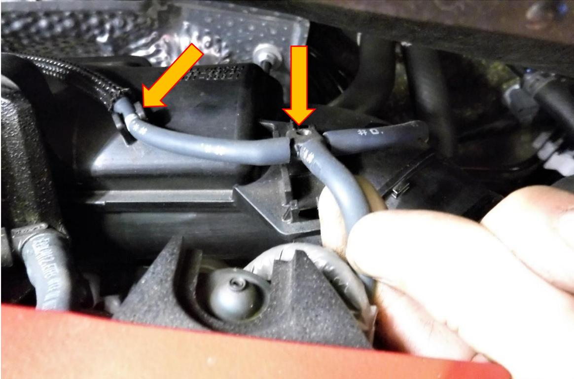
4. Using a 12mm socket and ratchet remove both M8 fasteners attaching the inlet hard pipe to the engine.
