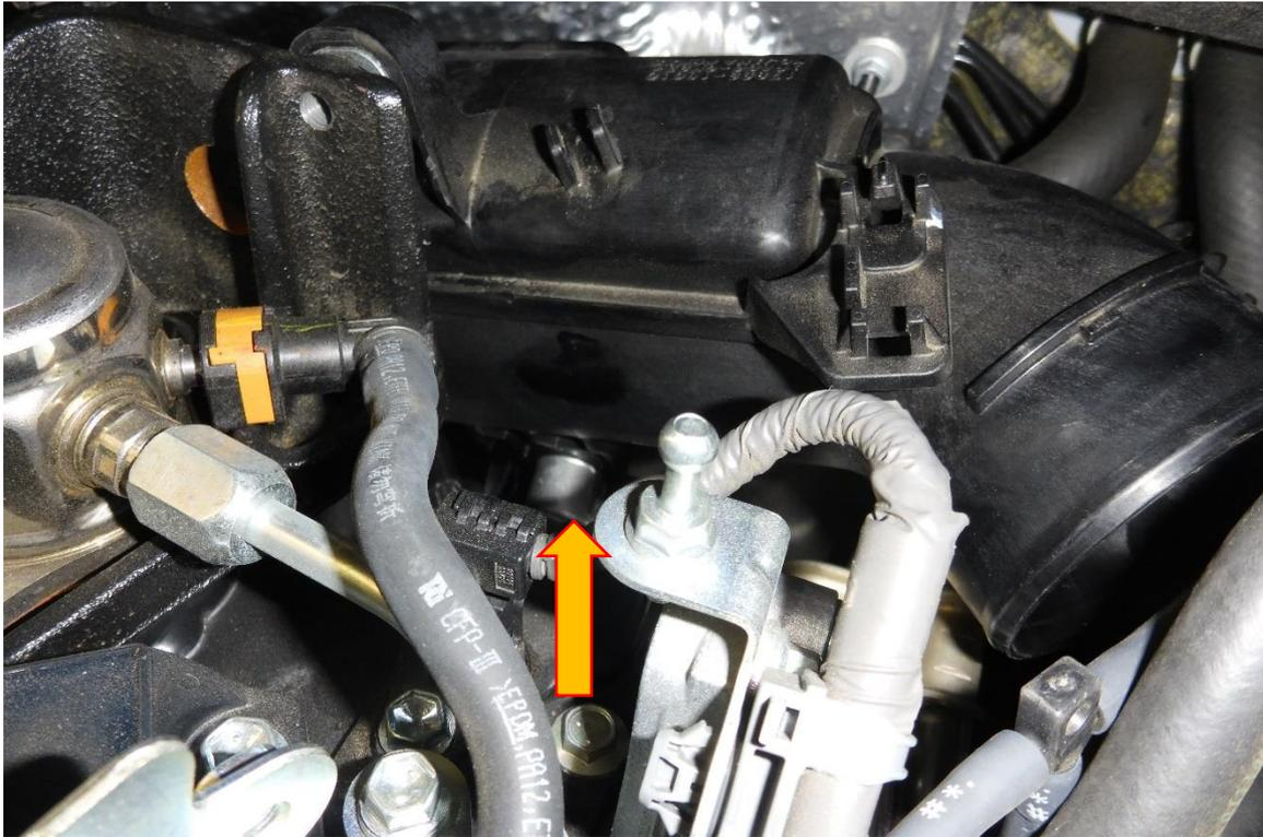
5. Using a 10mm socket and ratchet remove the M6 fastener further down on the underside of the hard pipe.
