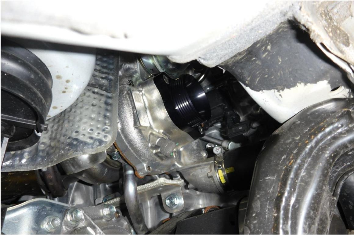
10. Take the silicone hose #2046 and fit it to the machined turbo adaptor. You will need to feed the silicone hose from the top of the engine bay down to the turbo, you may have to squeeze the silicone hose to get it past the heat shield. Secure the turbo end of the hose to the turbo adaptor using a 7mm socket and ratchet and supplied 50-70 hose clamp.
