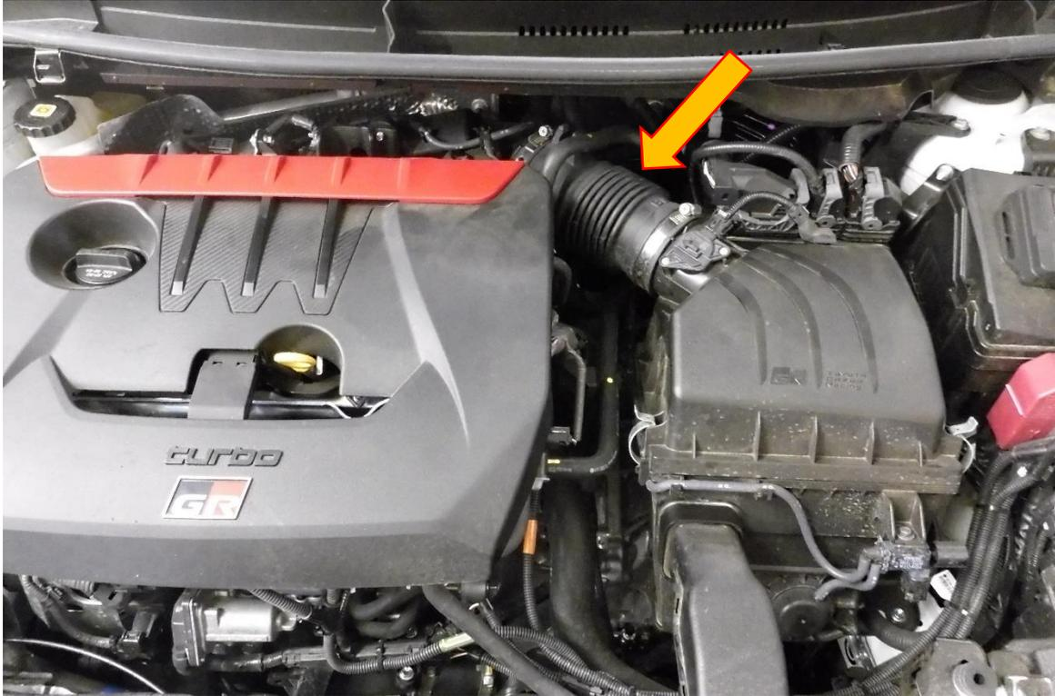
2. Using a 10mm socket and ratchet loosen both hose clamps attaching the OEM turbo inlet hose. The oil breather hose can will simply pull off to remove from situ.
