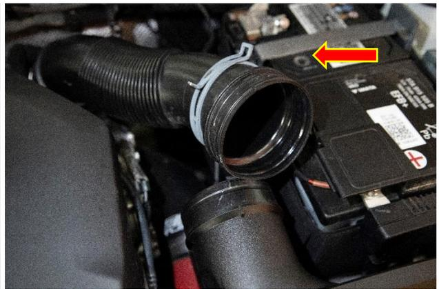
3. Using a 7mm socket or flat bladed screwdriver loosen the hose clamp and remove the hose from situ.
