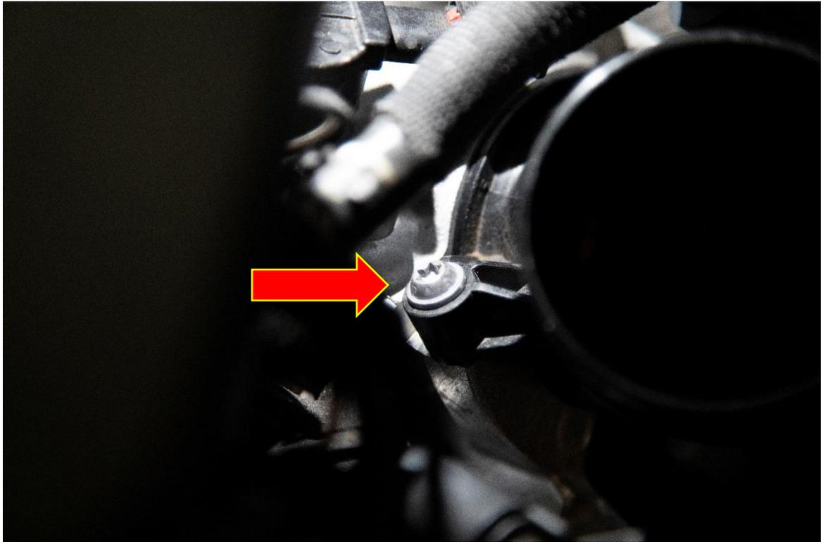
6. Rotate the elbow in a clockwise direction, the elbow can then be removed from situ.
