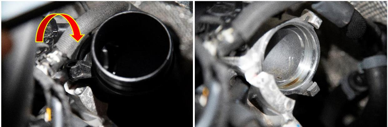
7. Remove the o-ring from the OEM elbow and fit onto the Forge Motorsport item as pictured below.
