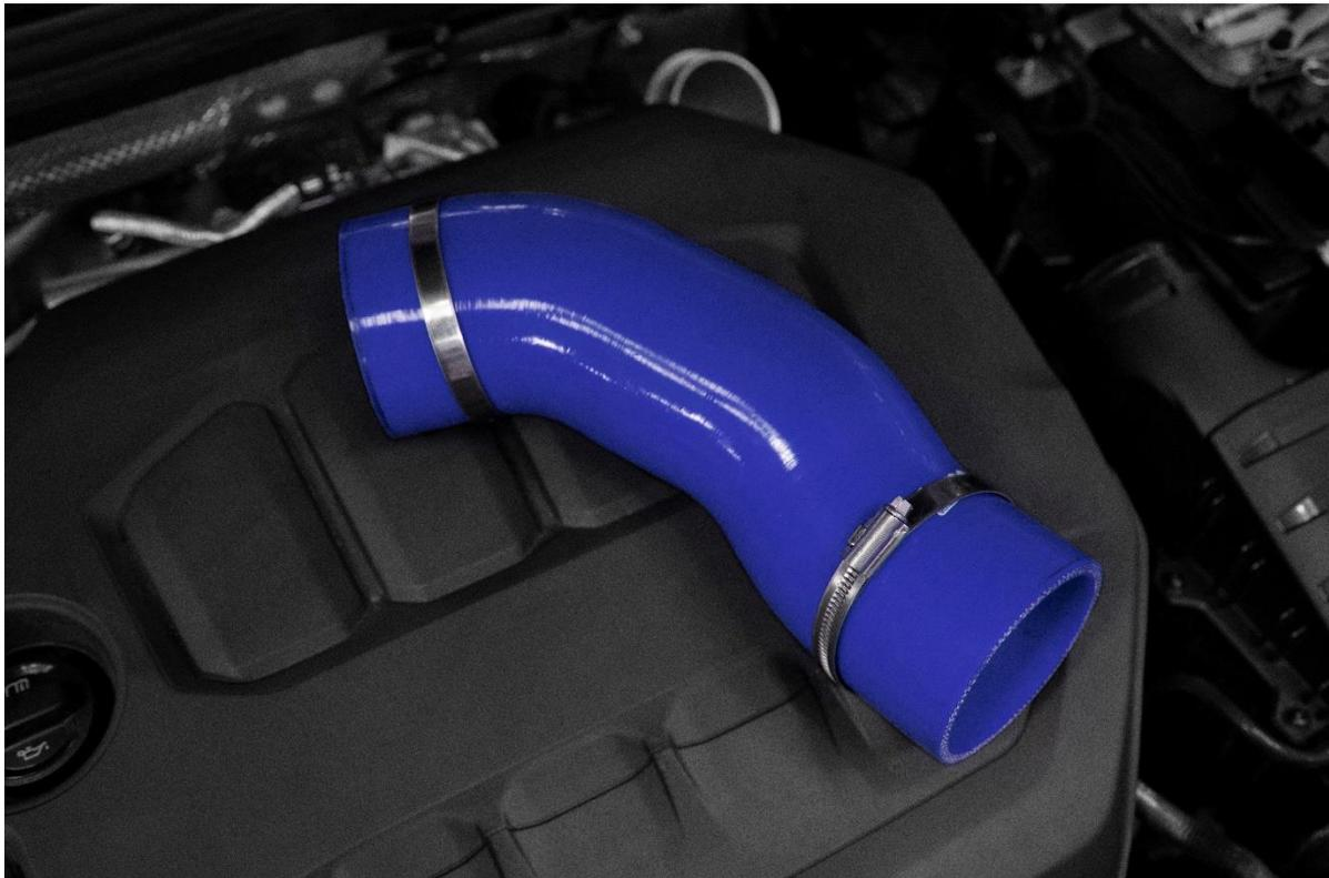
10. Fit the hose into position then using a 7mm hose clamp, tighten the junction at the turbo elbow end first.
