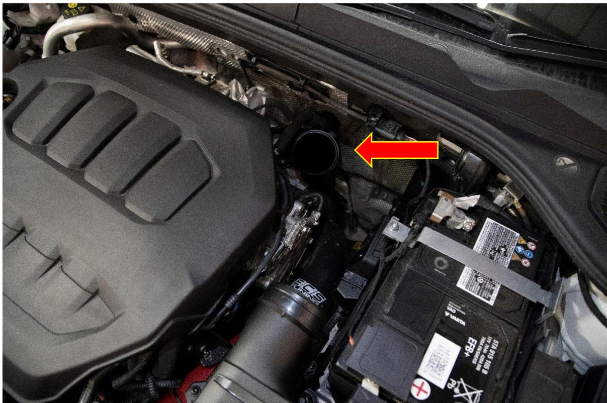
5. Using a T30 torx drive and suitable ratchet remove the fastener that holds the turbo elbow in position.
