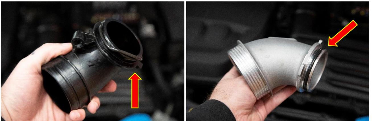
8. Fit the Forge Motorsport turbo elbow into position and rotate anti clockwise.
