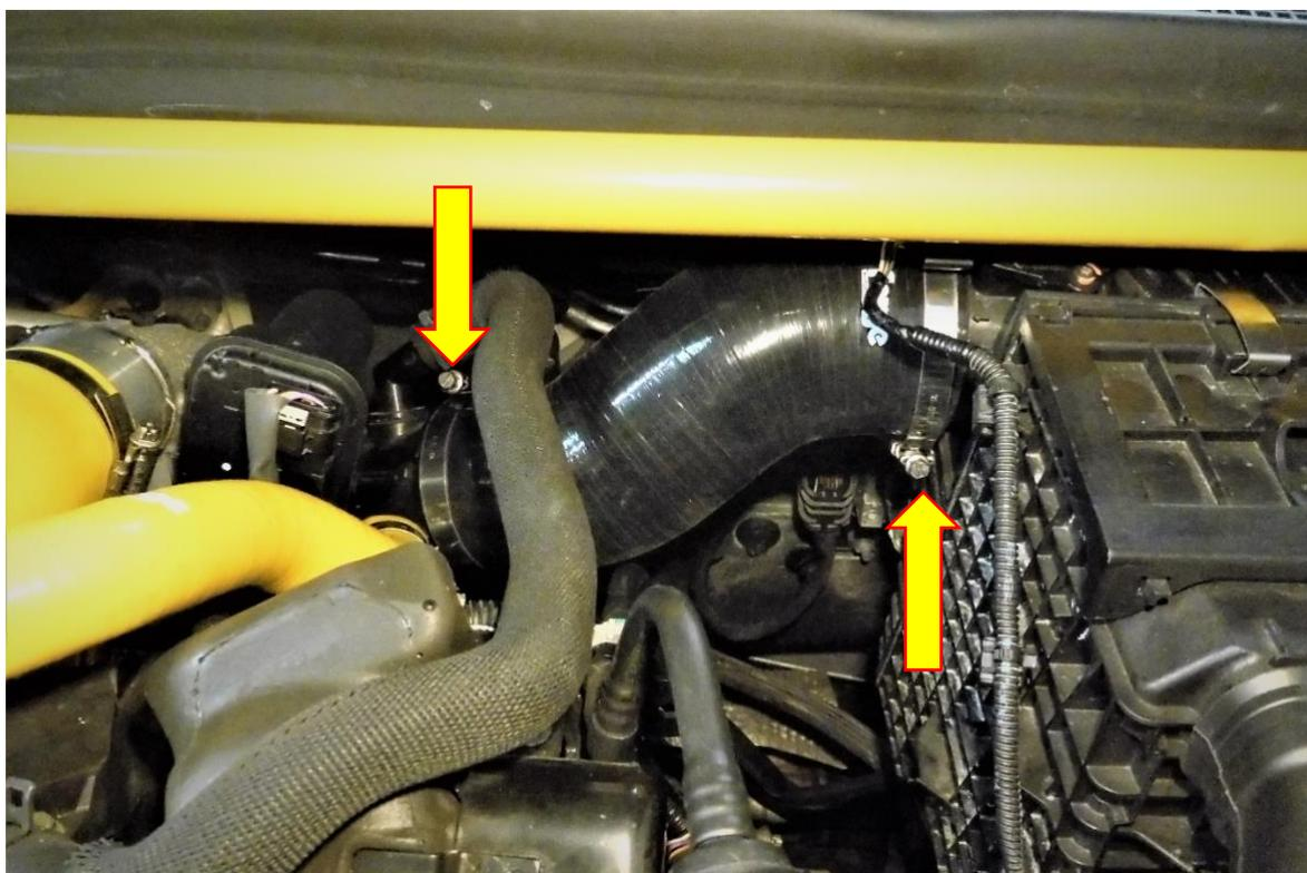
3. Using a hose removal tool remove the oil breather hose and the DV hose from the OR inlet elbow. With both hoses removed you will now be able to remove the turbo inlet hose from the vehicle.
