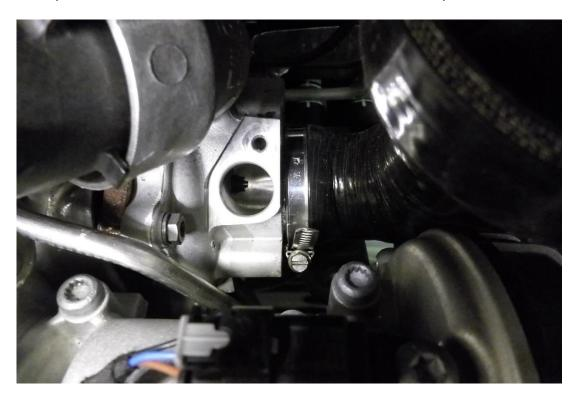
11. Re connect the breather pipes to the machined fittings on the FMTIA3 hose. And re fit the oil breather hose.
