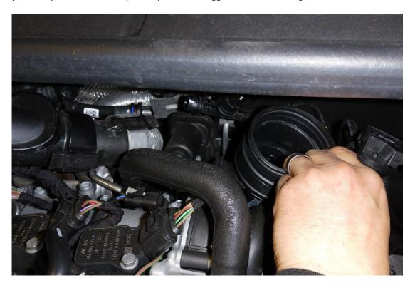
7. Depending on whether your vehicle has the extra breather system or not, the two pictures show which of the machined fittings should be attached to the FMTIA3 hose. Use both 12-22 hose clamps to secure the machined fittings.
