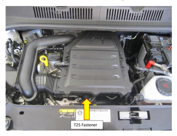
2. Remove the breather hose from the air box, this will just pull off. Next, remove the spring hose clamp with a hose removal tool or some pliers.
