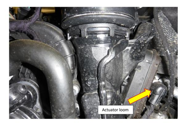
6. There is a hose attached to the underside of the turbo adaptor, these simply unclip. Now pull the OE turbo adaptor away from the turbo, you may have to wriggle it out as it is a tight fit.
