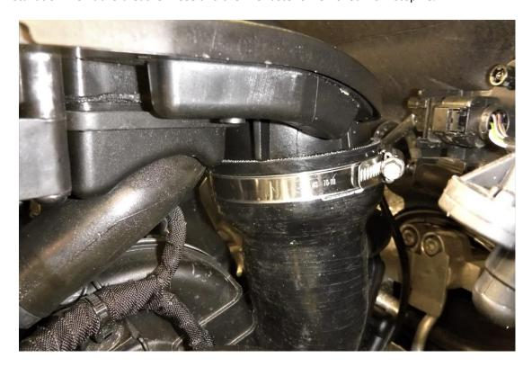
If you have a Forge Motorsport intake, fit and secure the alloy joiner to the induction hose first, then fit to the Forge FMTIA3.
