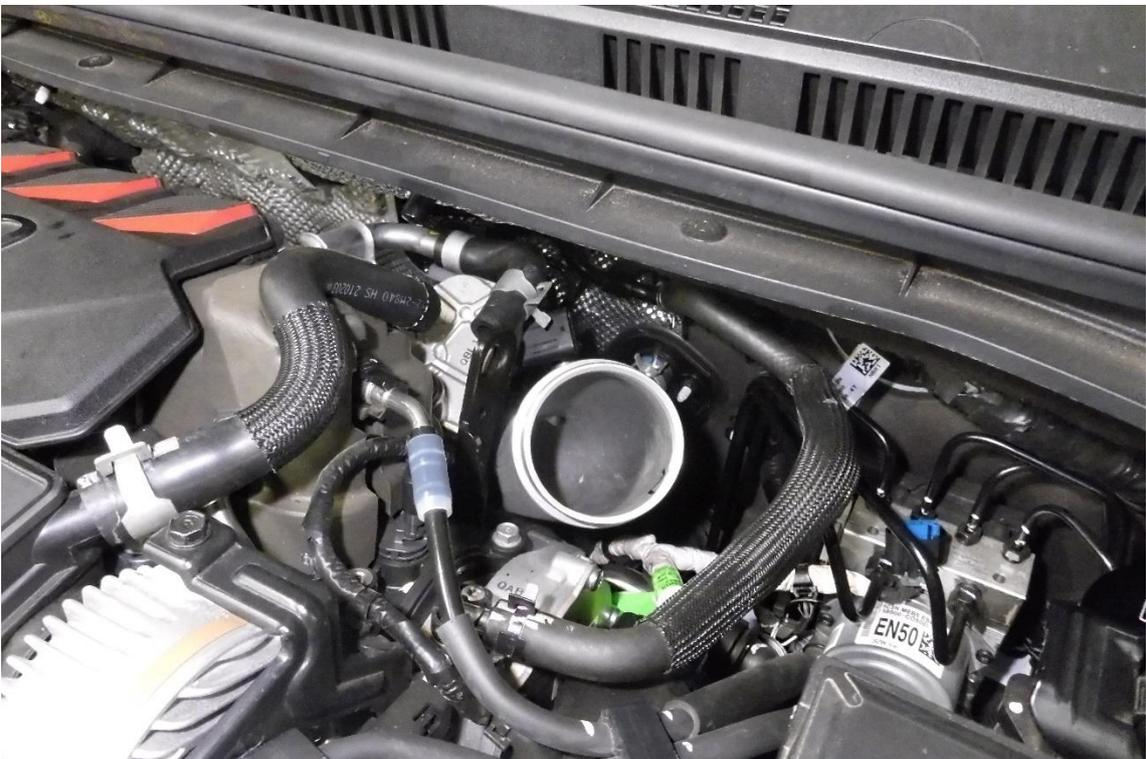
13. Re-attach the oil breather hose to the Forge Motorsport turbo adaptor and plug the wiring loom back into the turbo actuator.
