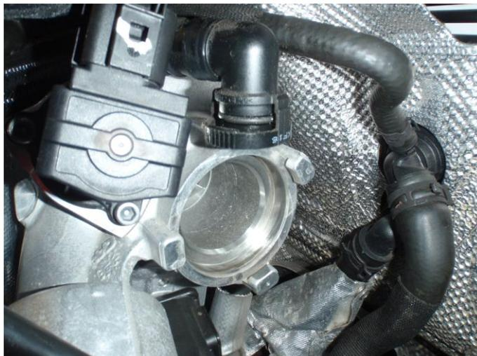
8. Rotate the turbo adapter until the correct alignment with the locking tabs is achieved. Push the coupler fully into the turbo inlet before rotating the part anti-clockwise.
