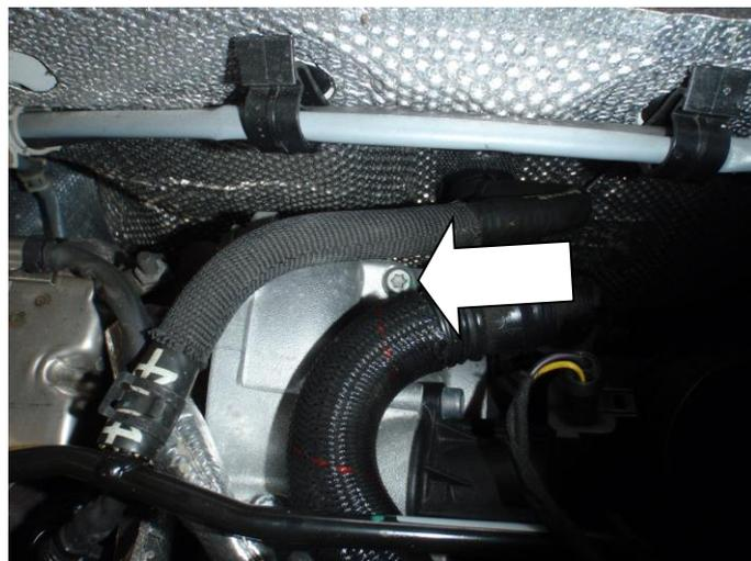
5. Rotate the plastic intake adapter toward the bulkhead to release it.
