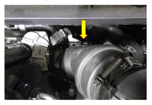
4. Using a flat bladed screwdriver prise the X2 plastic retaining clips open and remove them from the air duct.
