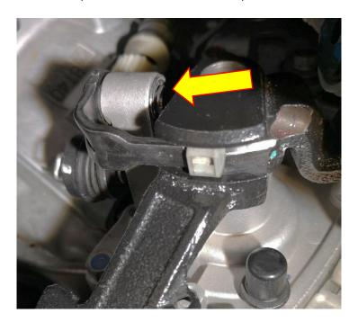
9. Take two flat head screwdrivers, place them on either end of the C-clip to pry it off the shaft. If you have a magnet, we recommend placing this behind the C-clip as it is very easy to drop this into the depths of the engine bay. When the C-clip is removed you can slide the mechanism out of the bore.
