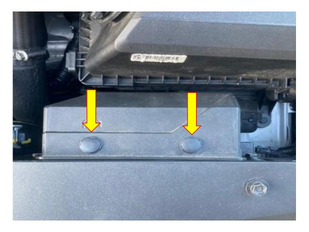
5. Using a 10mm socket and ratchet with extension remove the X3 M6 fasteners attaching the airbox to the vehicle. You will now be able to remove both the airbox and air duct from the engine bay.
