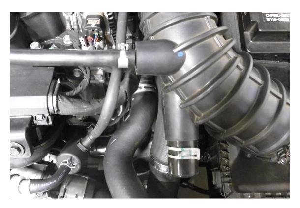
2. Using a 10mm socket and ratchet loosen the hose clamp attaching the inlet hose to the airbox, once loose detach it from the airbox-
