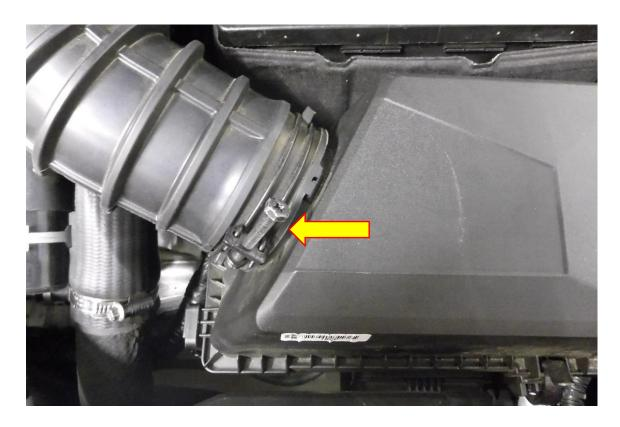
3. Again, using a 10mm socket and ratchet loosen the hose clamp and remove the opposite end of the inlet hose attached to the turbo adaptor. You can now remove the hose completely.
