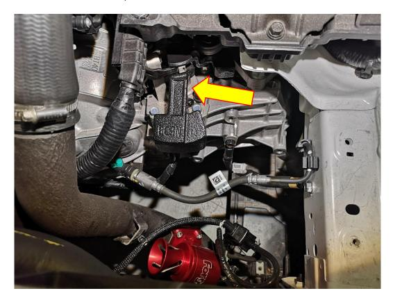
7. Pull the R clip out of the shifter cable labelled below, this will allow you to unclip the shift cable from the OEM shifter. The supplied circular clip will be used for reassembly of the Forge Motorsport short shifter.
