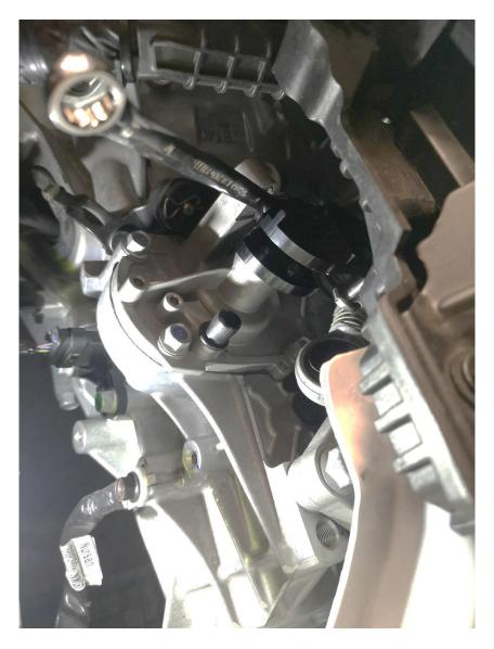
**15**. Move the pin into the desired position and tighten with a 16mm spanner, the longest shift length is the same as the OEM shift length.
