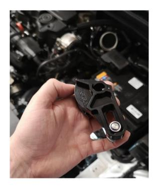
13. Fit the Forge Motorsport short shifter over the shaft, and fit the 30mm hex head bolt and nyloc nut in the orientation as shown below (nut fits into the groove inside the short shifter)
