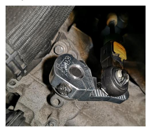
10. You have now successfully installed your Forge Motorsport short shifter, perform a final spanner and connections check. Now take your vehicle for a test drive and enjoy your new Forge Motorsport product.
