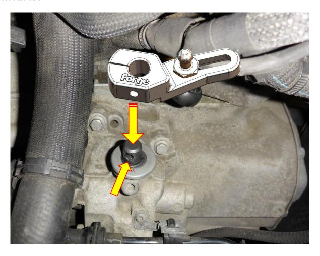
8. Using a 10mm socket and suitable driver and a 10mm spanner attach the supplied M6 bolt, washers and nyloc nut through the hole in the shifter and shaft to secure the shifter as detailed below.
