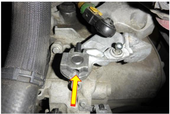
7. Fit the ball pin to the Forge short shifter as illustrated below in step 8. Using a 16mm spanner tighten the ball pin in desired position along the adjustment slot. Take the Forge Motorsport Short shifter and place it onto the shaft, lining up the hole labelled below with the hole in the short shifter shaft. The orientation is illustrated below.
