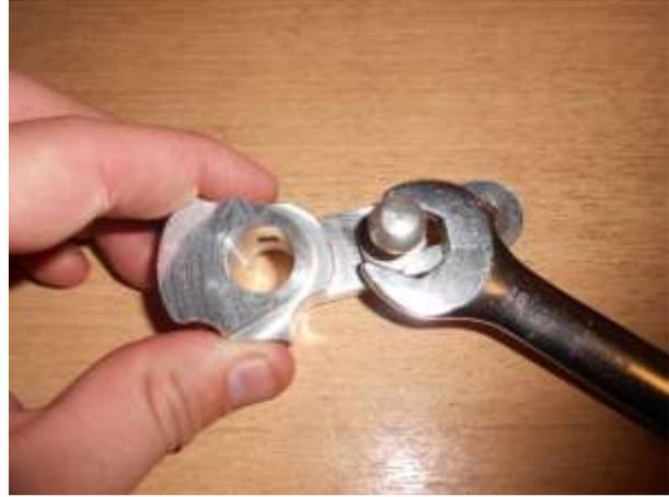
12. Secure your Forge quickshifter in position using the split pin supplied. Ensure the up and down shift arm is correctly located. Start the split pin on a solid surface before fitting in to the gearbox shaft.
