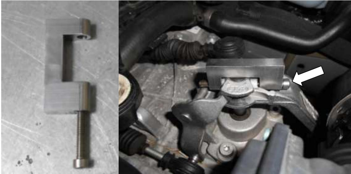
10. Carefully pull the shift arm upwards to remove it.
