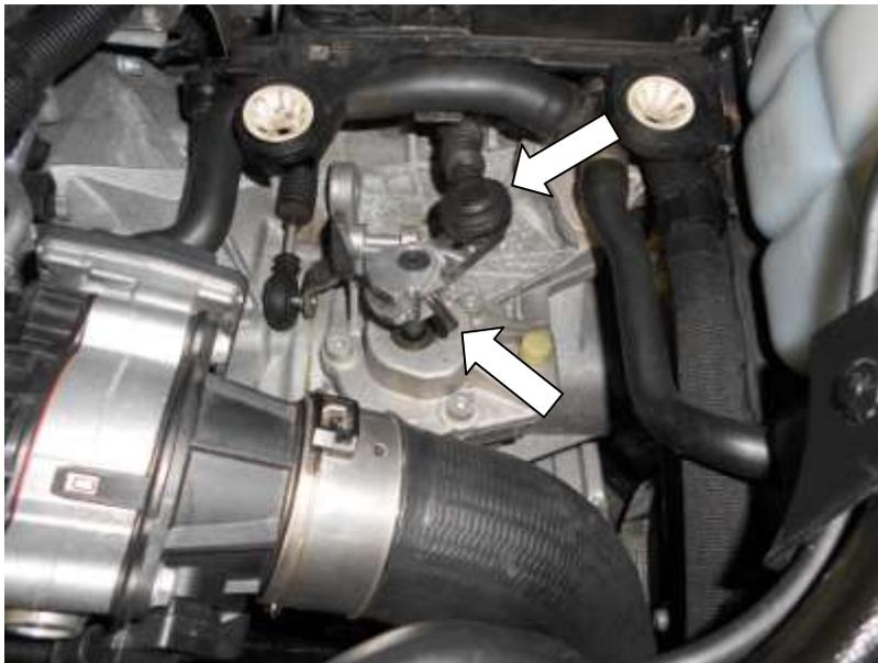
13. Using a hammer and drift or G-clamp push the split pin fully into the quickshifter body and reconnect the shift cable ball joint.
